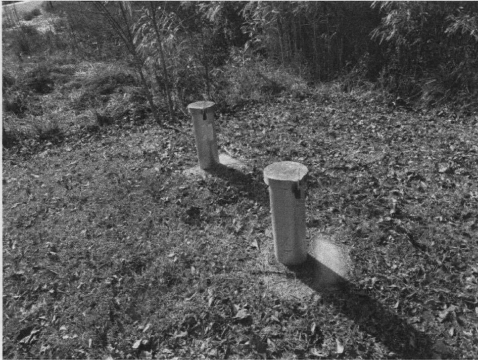
Monitoring wells FL-01-1 and FL-01-2 are located outside of the landfill fence. The wells were locked and appeared to be in good condition.
