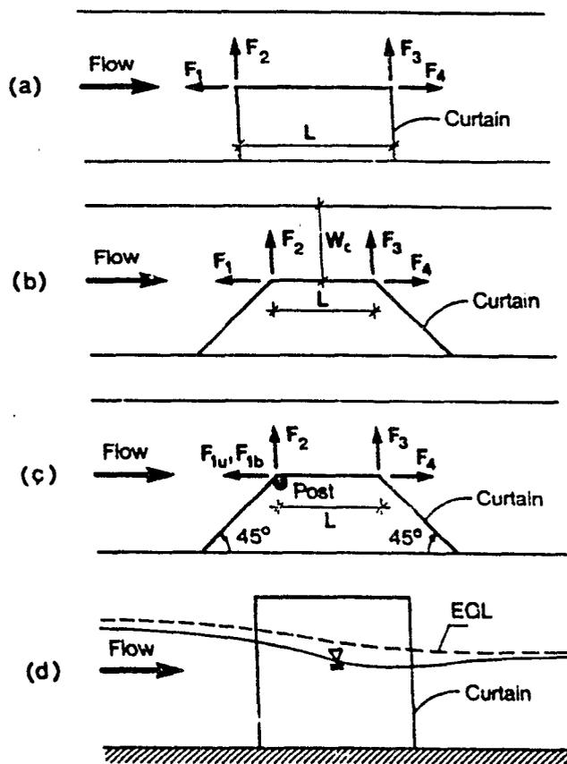
Figure 2 - Schematic of silt curtain layout
