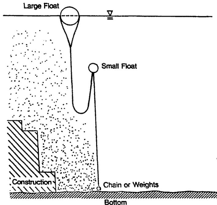
Figure 5 - Cross section of a 2-float curtain
