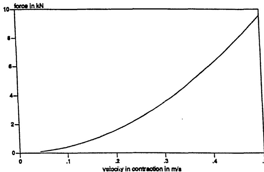
Figure 3 - Example of total force as a function of velocity
