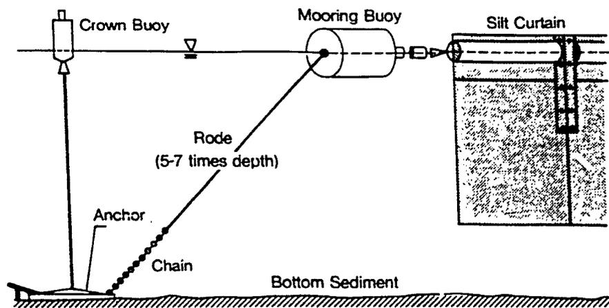
Figure 1 - Recommended mooring system for silt curtains (Barnard, 1978)
