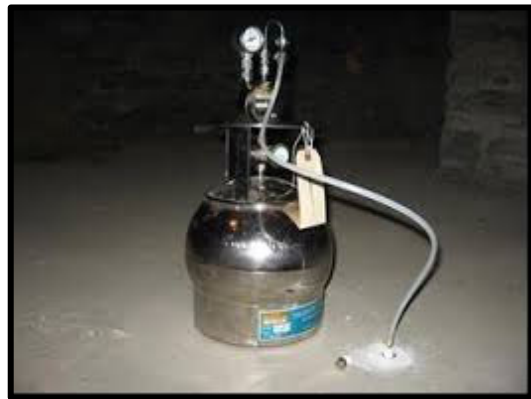
Sub-slab Sample Setup (summa canister connected to sub-slab sample port)
