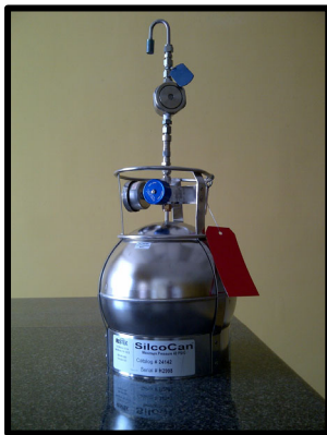
Indoor Air Sample Setup (summa canister on table)
