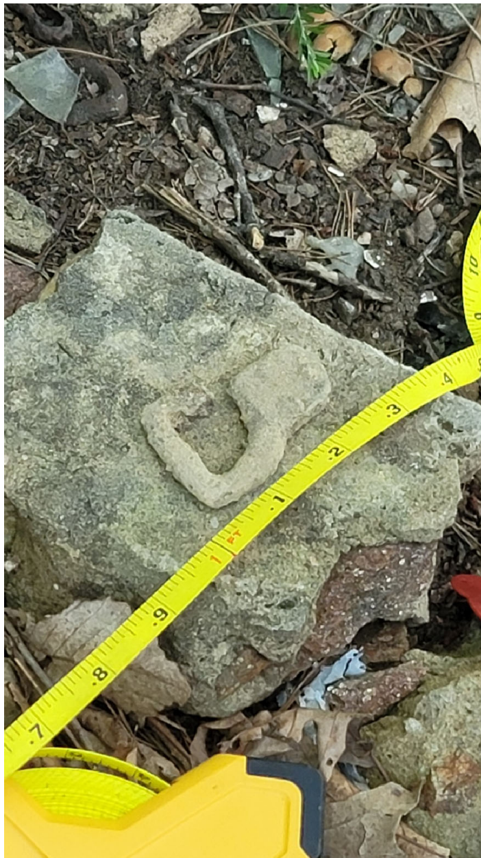
Attachment 2: Metal object (hook) emitting orders of magnitude above background radiation found after digging one foot of soil on-Site.
