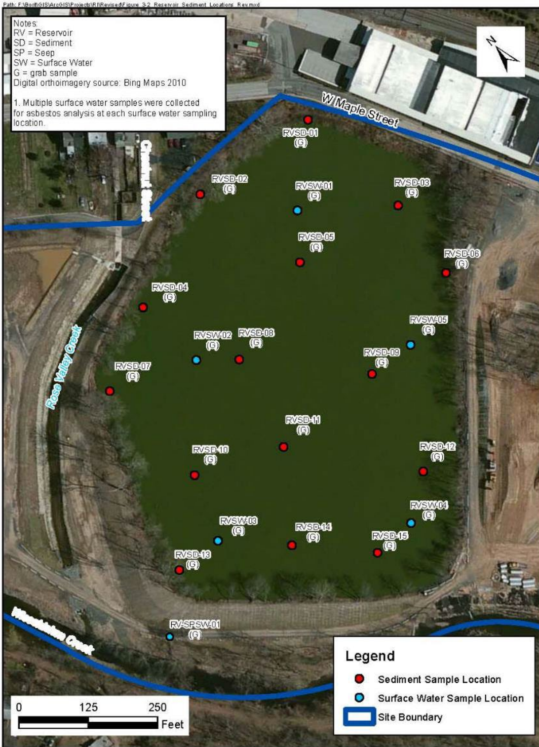
Figure 3-2 Reservoir Sediment, Surface Water, and Seep Sample Locations
