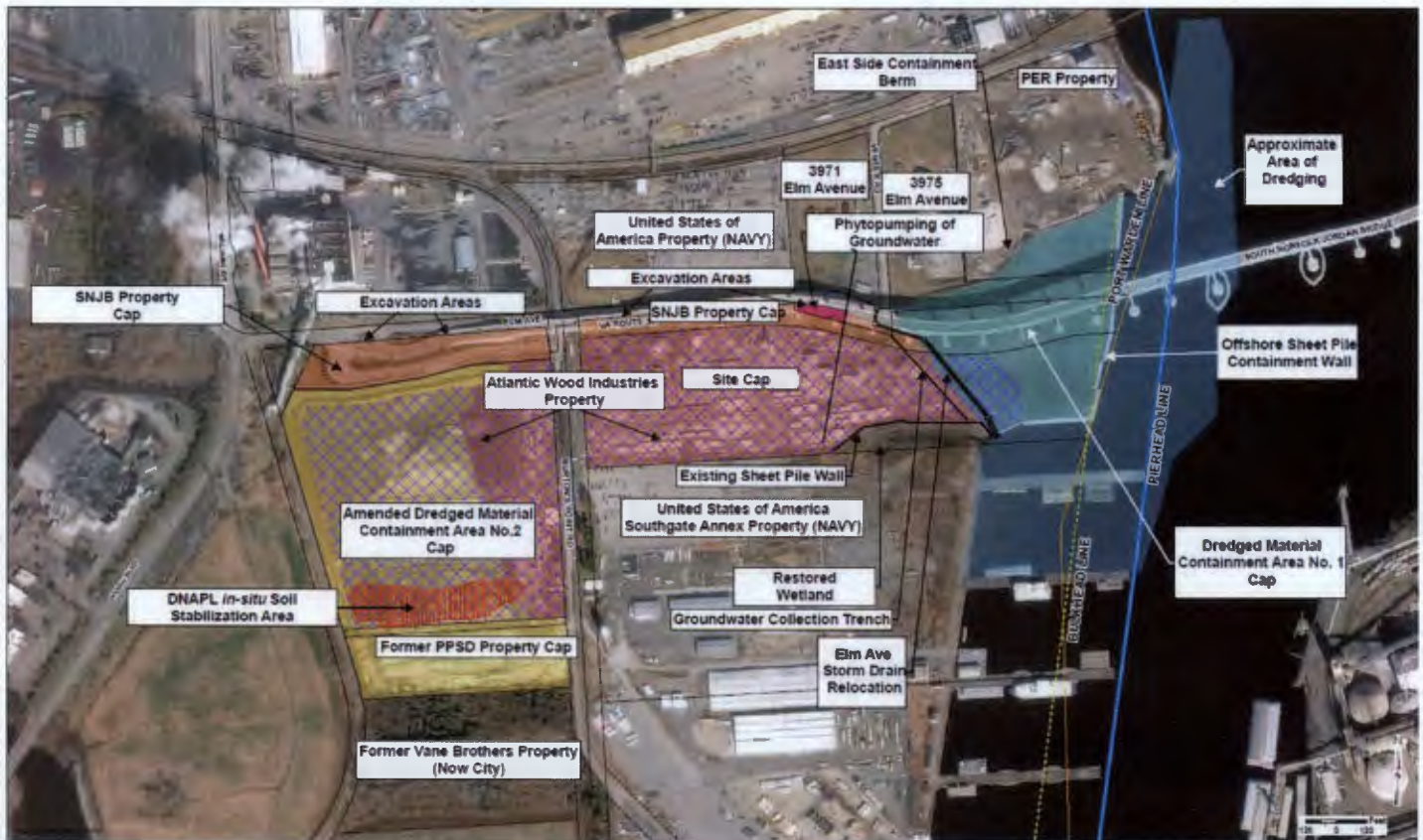
Figure 1: AWI Site showing elements of the cleanup and properties at or near the Site.
