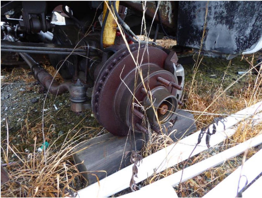
Scrap vehicle stored on SBA with proper use of wood to prevent cap damage
