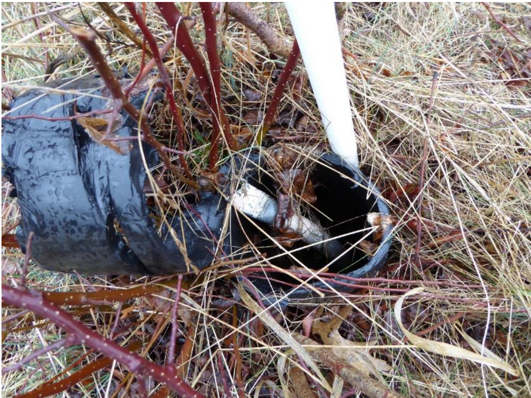
Damaged settlement monument on Inert Area, resurveyed in 2010
