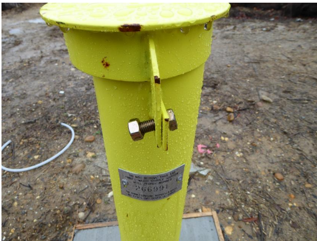
Unsecured monitoring well UPA-109. A lock was added after the inspection.
