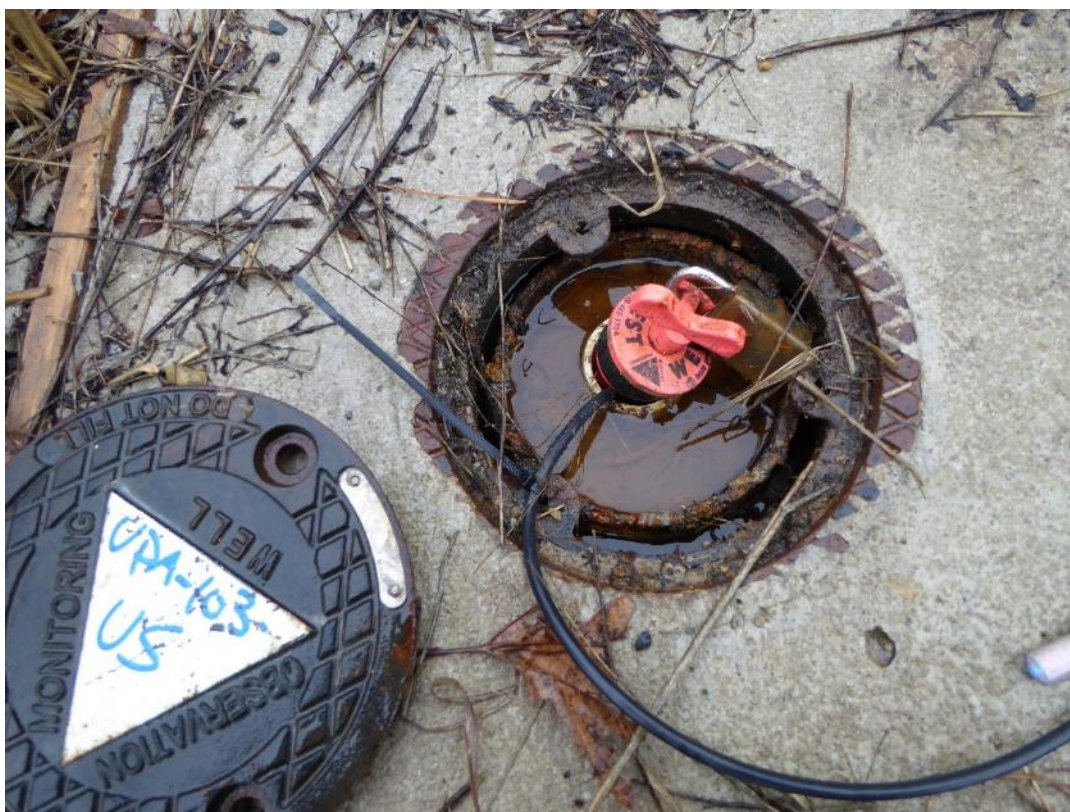
Monitoring well UPA-103-US left unsecured for water level monitoring, with rainwater collecting
