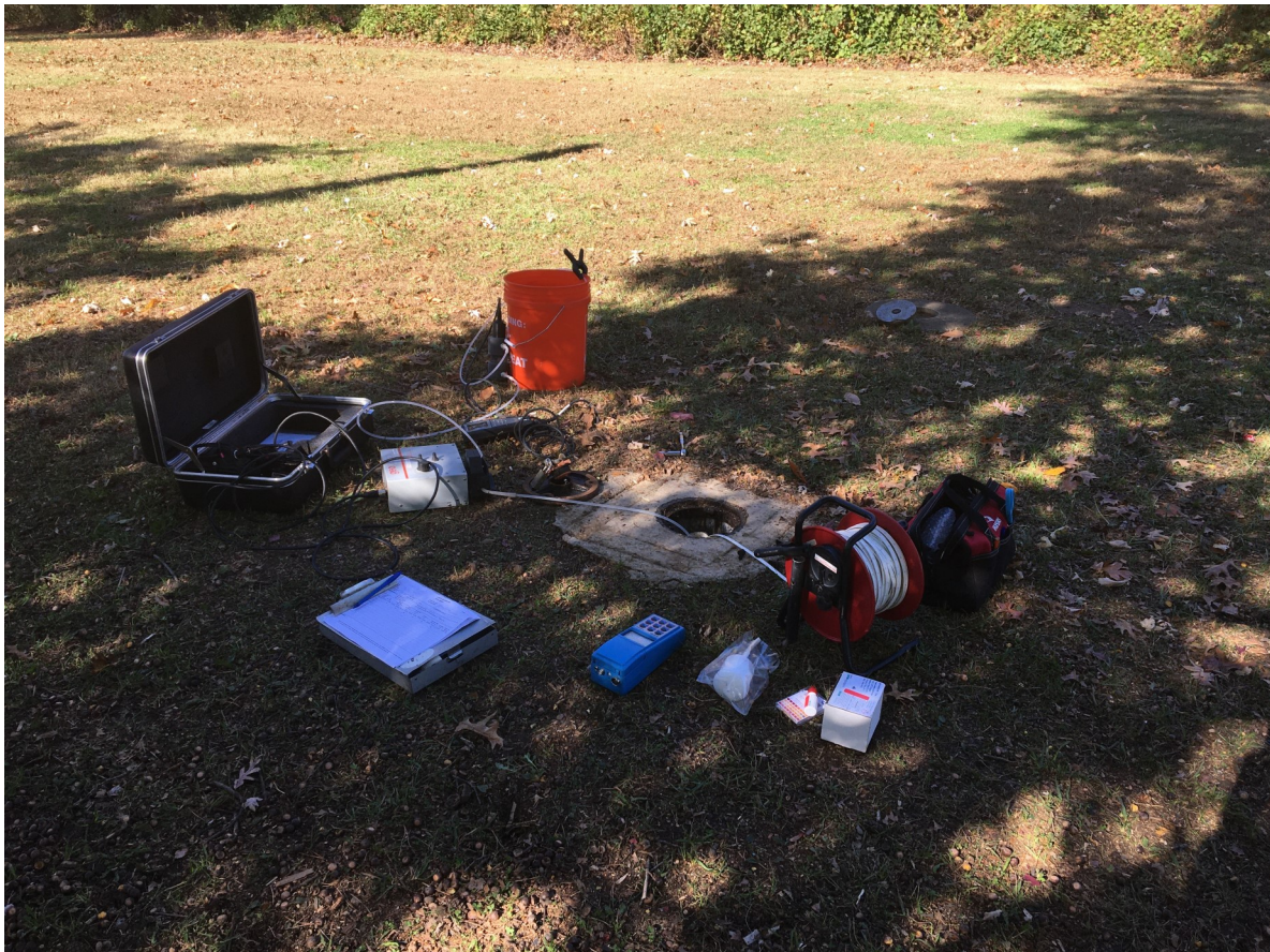
Example of groundwater sampling and equipment near the Havertown PCP Superfund Site.
