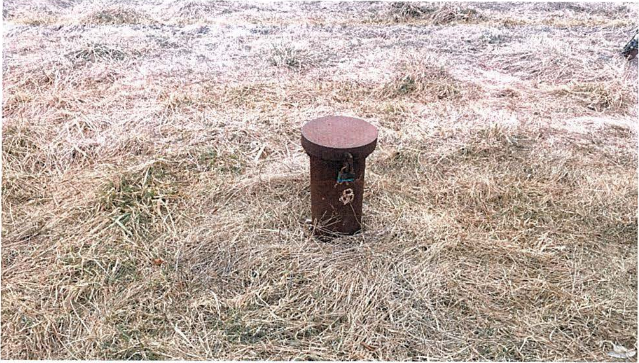
Picture 3. Monitoring well (MW-008).
