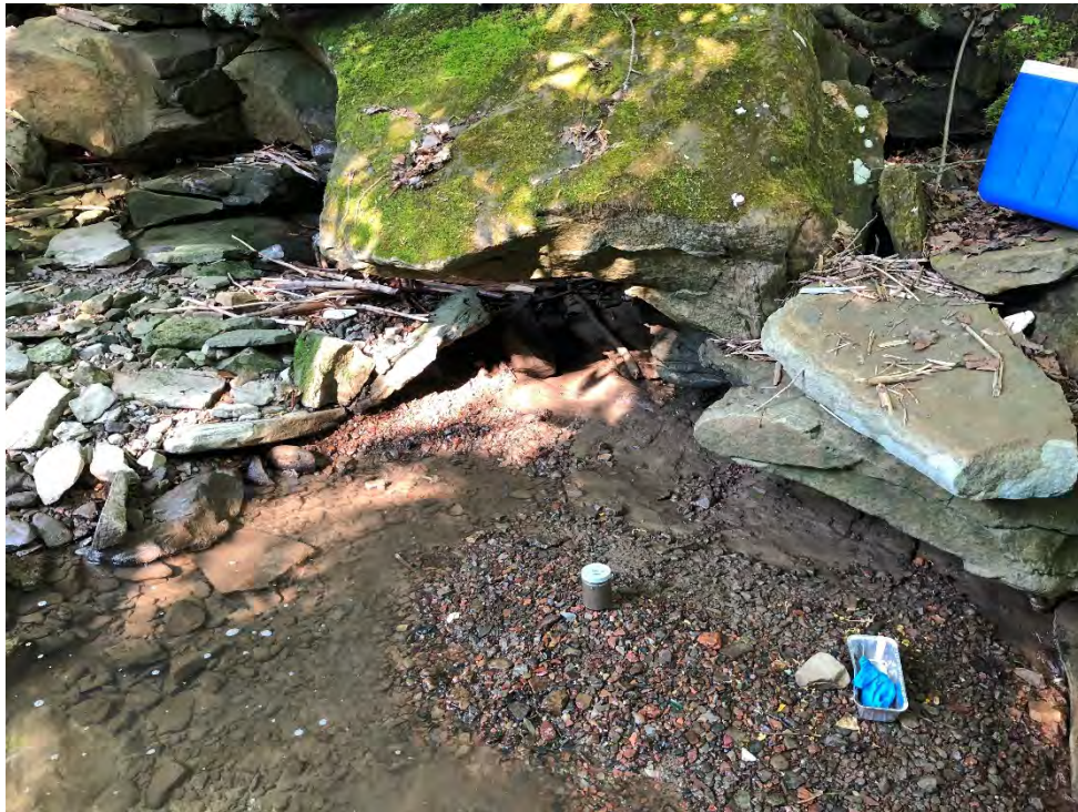
Photograph Description: SEC-SD-56; Sediment collected from west bank of Arbuckle Creek. Sediment is silty, medium-coarseness. Creek fauna (salamander and crawfish) observed at sampling location. Date: 15 May 2018
