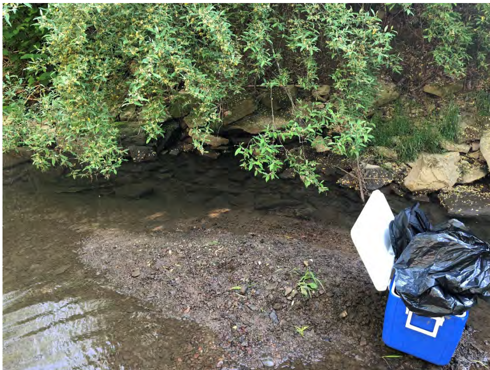
Photograph Description: SEC-SD-57; Sediment collected from east bank of Arbuckle Creek. Sediment is gravelly with sand and some silt; coarse grain. Date: 15 May 2018
