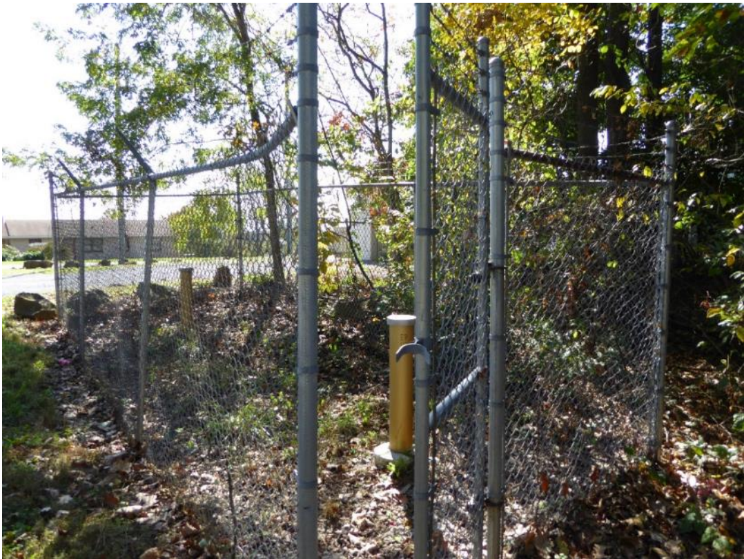
Monitoring well EP02, near entrance to site property. Gate is not locked.
