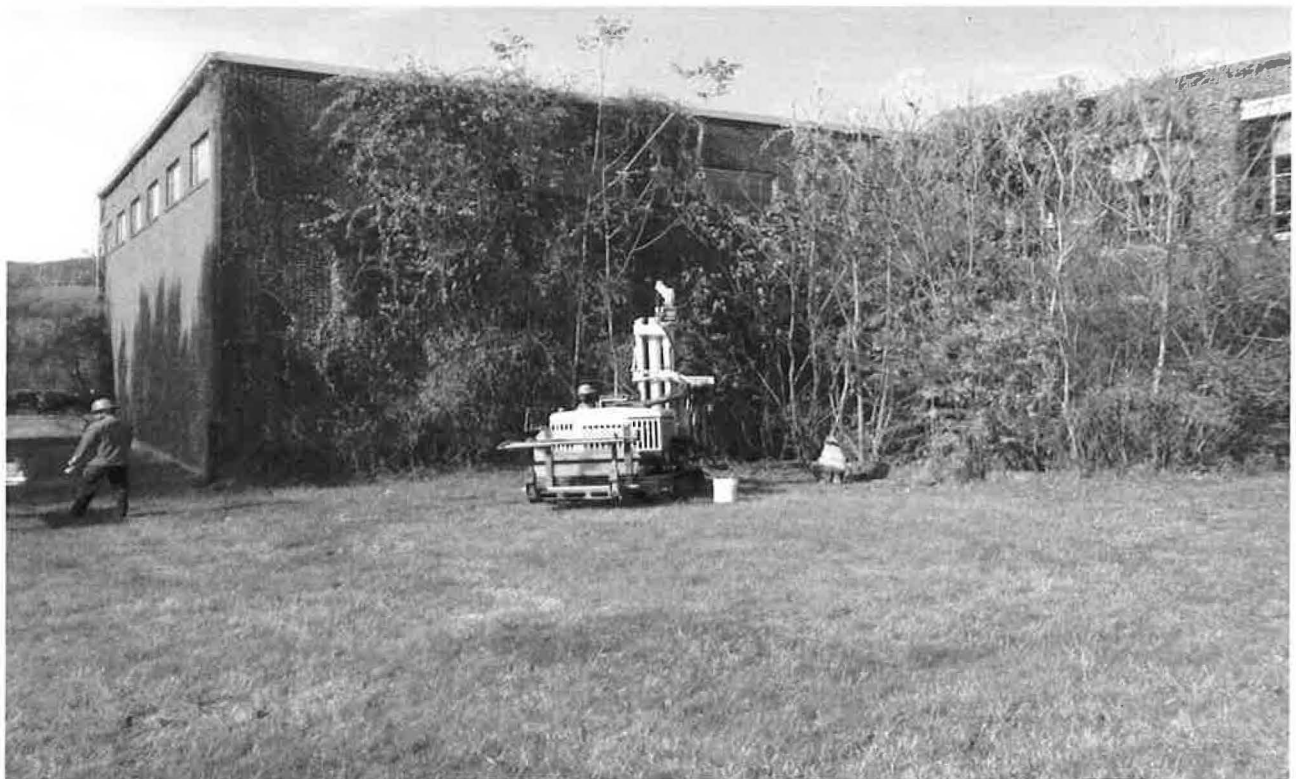
Hellertown Manufacturing Co. Superfund Site - Fourth Five-Year Review Geoprobe in Former Underground Storage Tank Area
