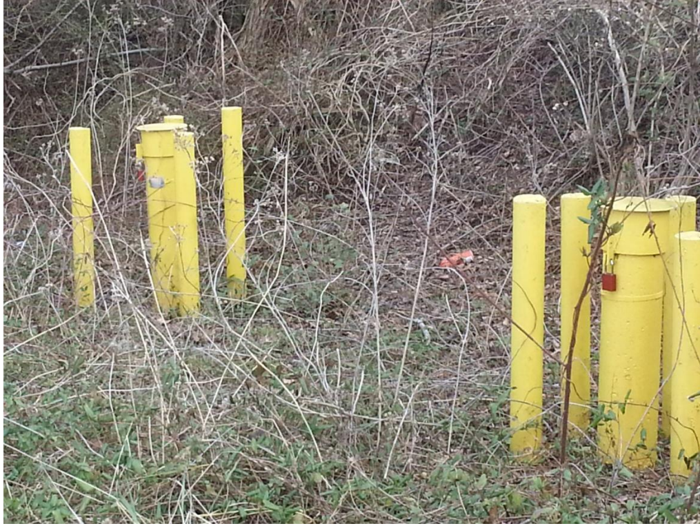
New locks installed on GW monitoring wells MW-07A and MW-07B during 2-27-13 site visit.
