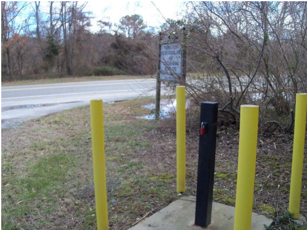
New lock installed on LFG monitoring well 1-GW6 during 2-27-13 site visit.
