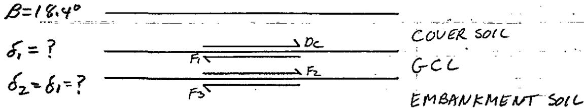
FOR A FACTOR OF SAFETY OF 1.5 FOR THE INTERFACE BETWEEN THE GEOSYNTHETIC CLAY LINER WITH THE COVER SOIL OR THE EMBANKMENT SOIL AN INTERFACE FRICTION ANGLE,  $\delta_1$  &  $\delta_2$  MUST BE DETERMINED
