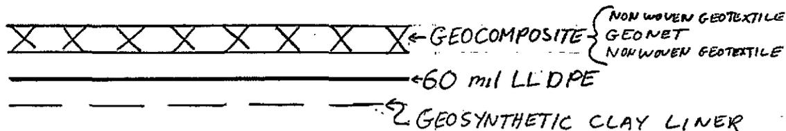
GEOSYNTHETIC INTERFACE FRICTION
