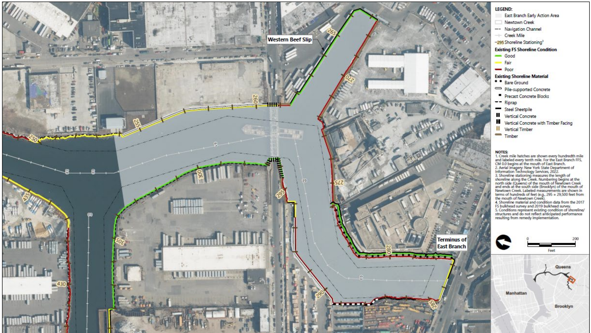
Figure 3 – Existing Shoreline Conditions East Branch
