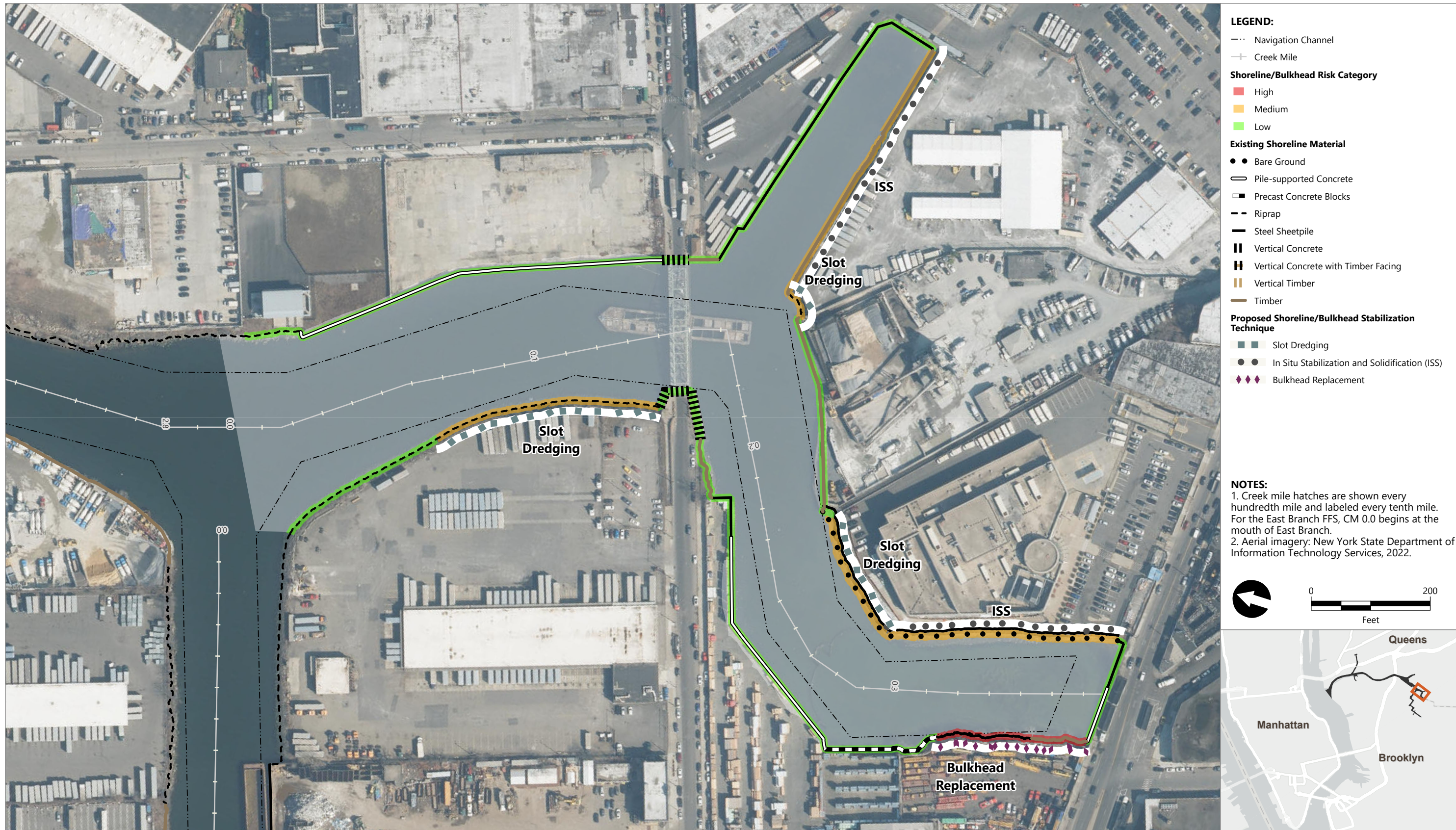
Figure E5-2 Shoreline/Bulkhead Risk Category and Proposed Shoreline/Bulkhead Stabilization Technique: Alternative EB-B
