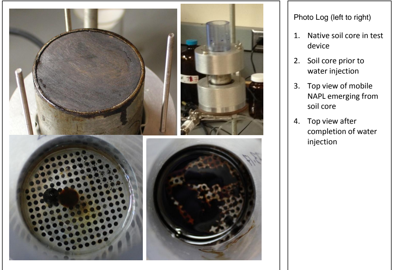
Figure 5: Native soil core segment is held in device that allows water to be pushed upward through the core resulting in NAPL migration (dark brown material in the photo) at start and end of test.
