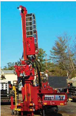
Drill rig used to collect soil
