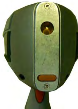
Figure 2-5. View of Face Plate and measurement window
