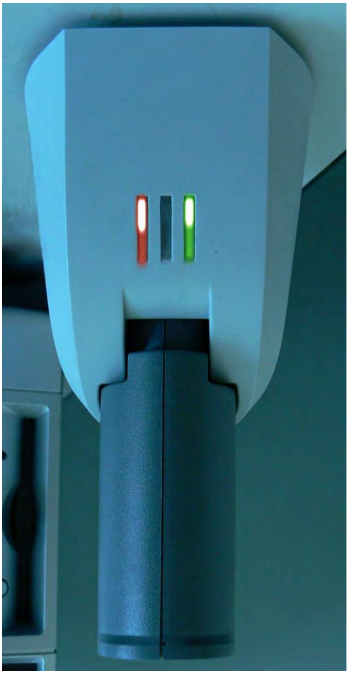
Figure 2-4. Battery Pack in the Charger
