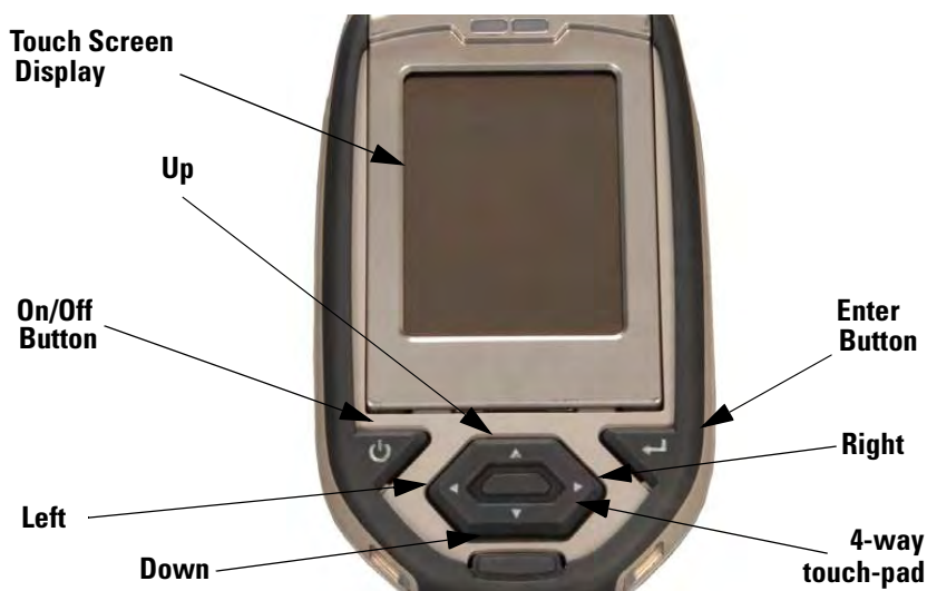
Figure 1-3. The Control Panel
