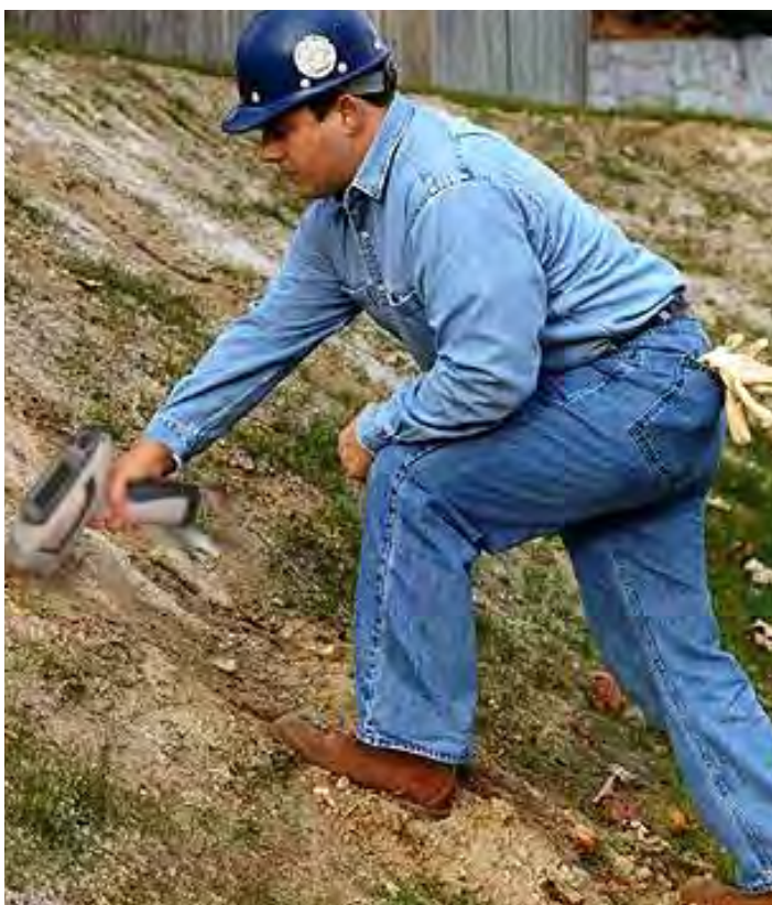
Figure 1-1. In-Situ Soil Testing
