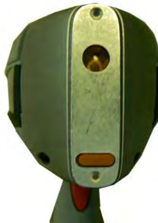
Figure 2-7. Fitting Face Plate over Proximity Button
