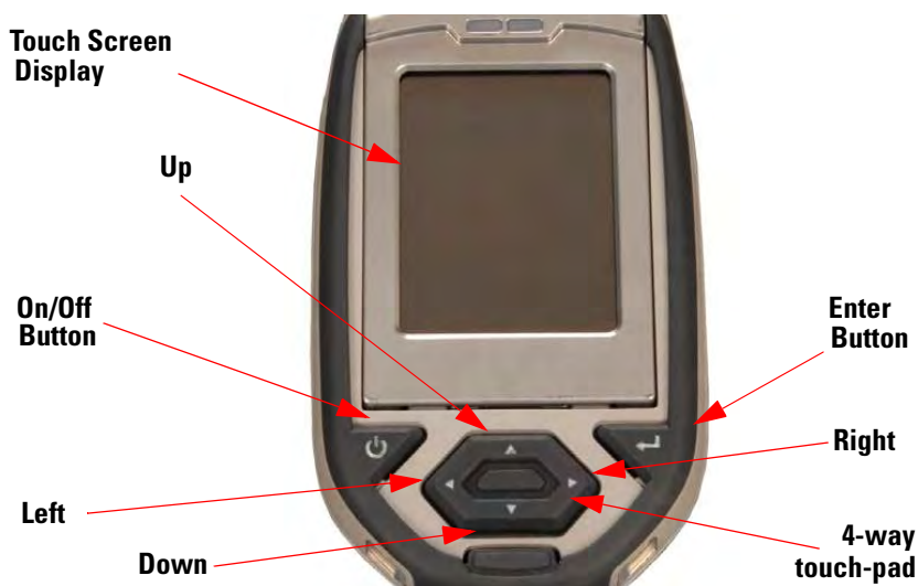
Figure 1-7. The Control Panel
