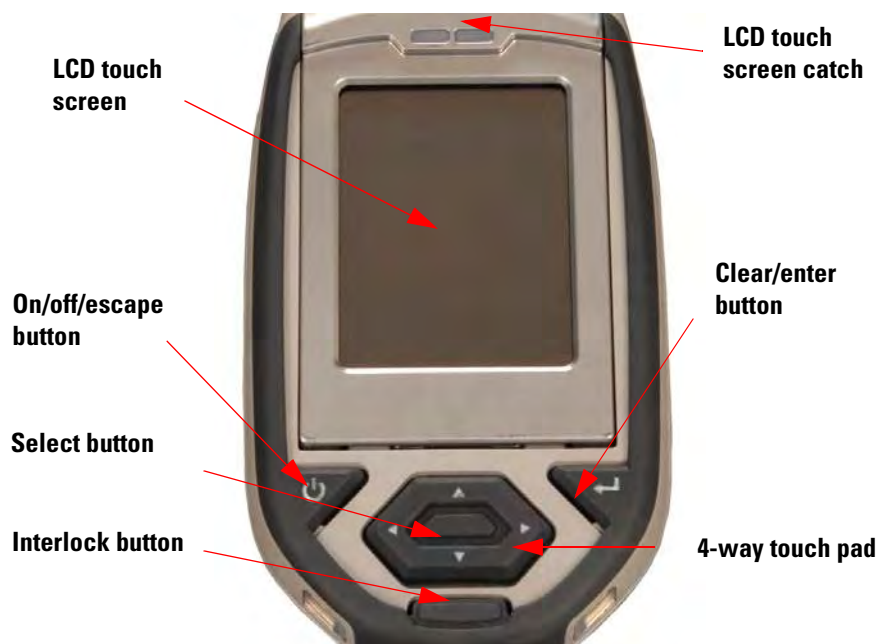
Figure 0-2. The Control Panel
