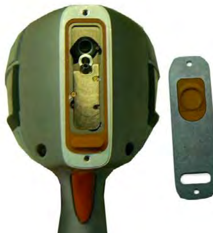
Figure 2-6. Face Plate Removed showing measurement window on Reverse
