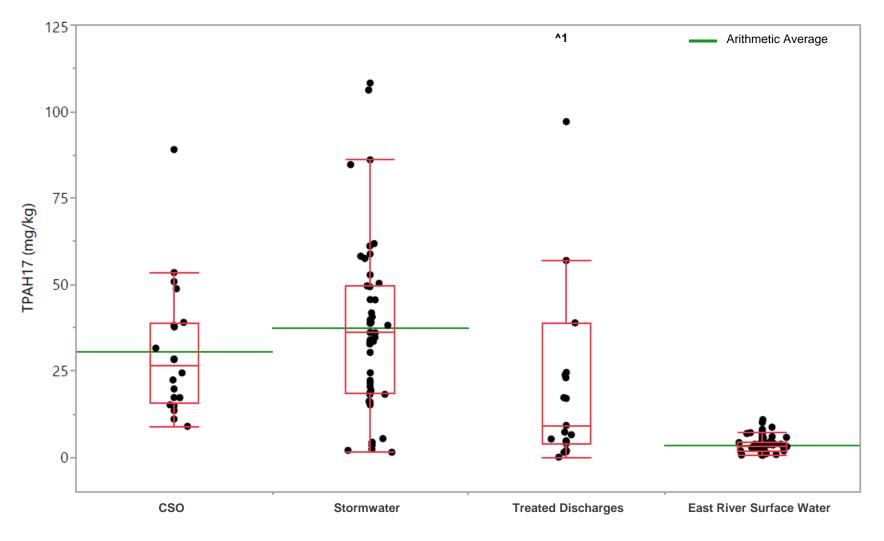
Note: Average concentration of TPAH17 in treated discharges is 2,056 mg/kg, which is outside the scale of the figure.
