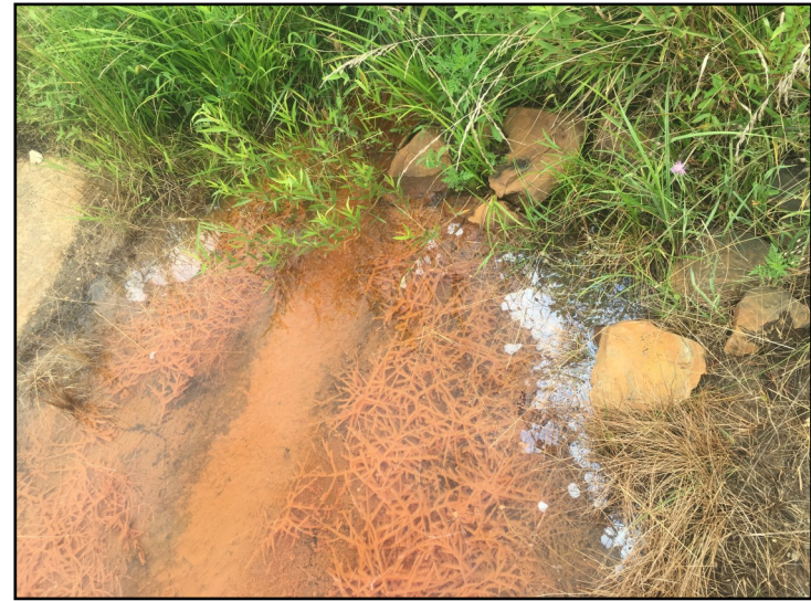
Photo 8. View of seep discharge at drainage channel crossing, note sheen and orange/oxidization.
