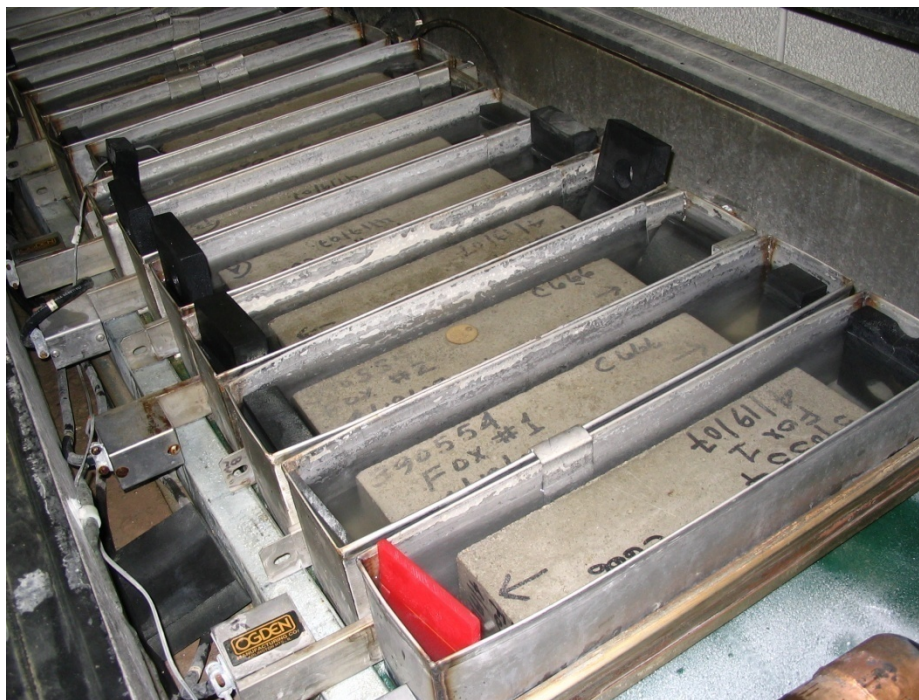
Figure 5. Concrete Blocks of Ecomelt-Based Blended Cement Being Subjected to Freeze-Thaw Cycles at CTLGroup Laboratories
