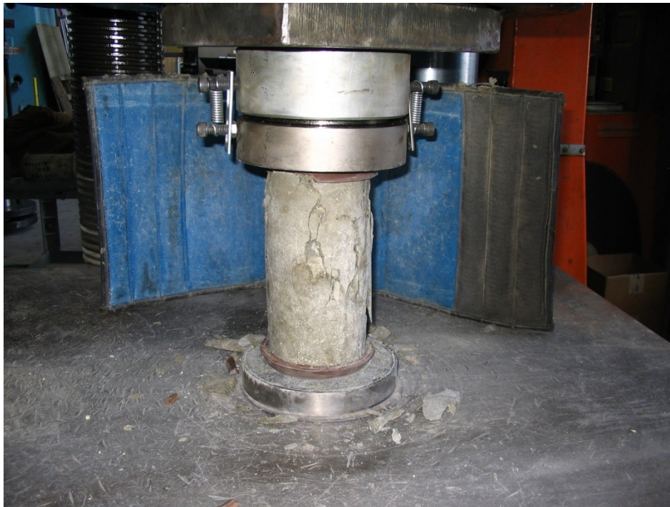
Figure 2. Concrete Cylinder of Ecomelt-Based Blended Cement After Compressive Strength Testing at CTLGroup Laboratories
