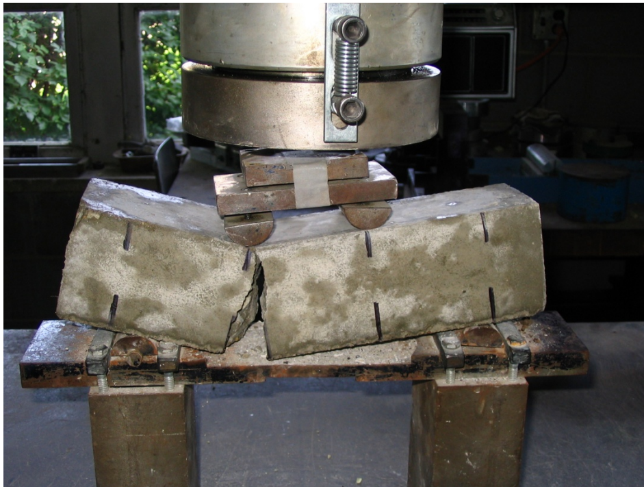
Figure 4. Concrete Block of Ecomelt-Based Blended Cement After Flexural Strength Testing at CTLGroup Laboratories
