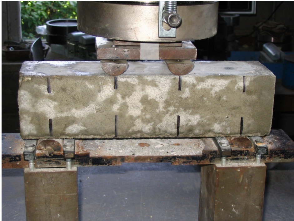
Figure 3. Concrete Block of Ecomelt-Based Blended Cement in Position for Flexural Strength Testing at CTLGroup Laboratories
