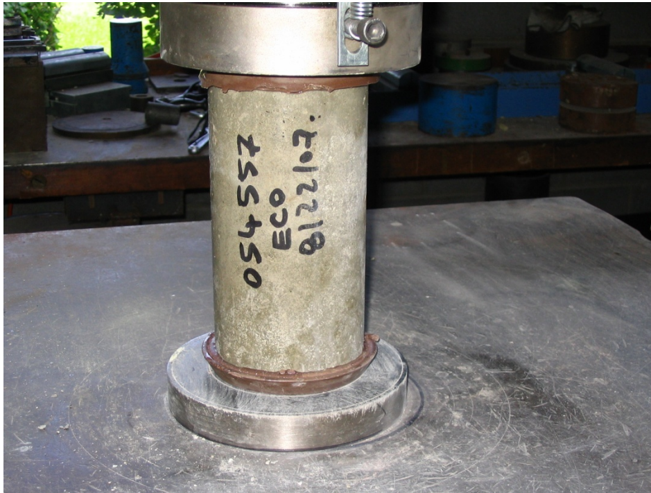
Figure 1. Concrete Cylinder of Ecomelt-Based Blended Cement in Position for Compressive Strength Testing at CTLGroup Laboratories
