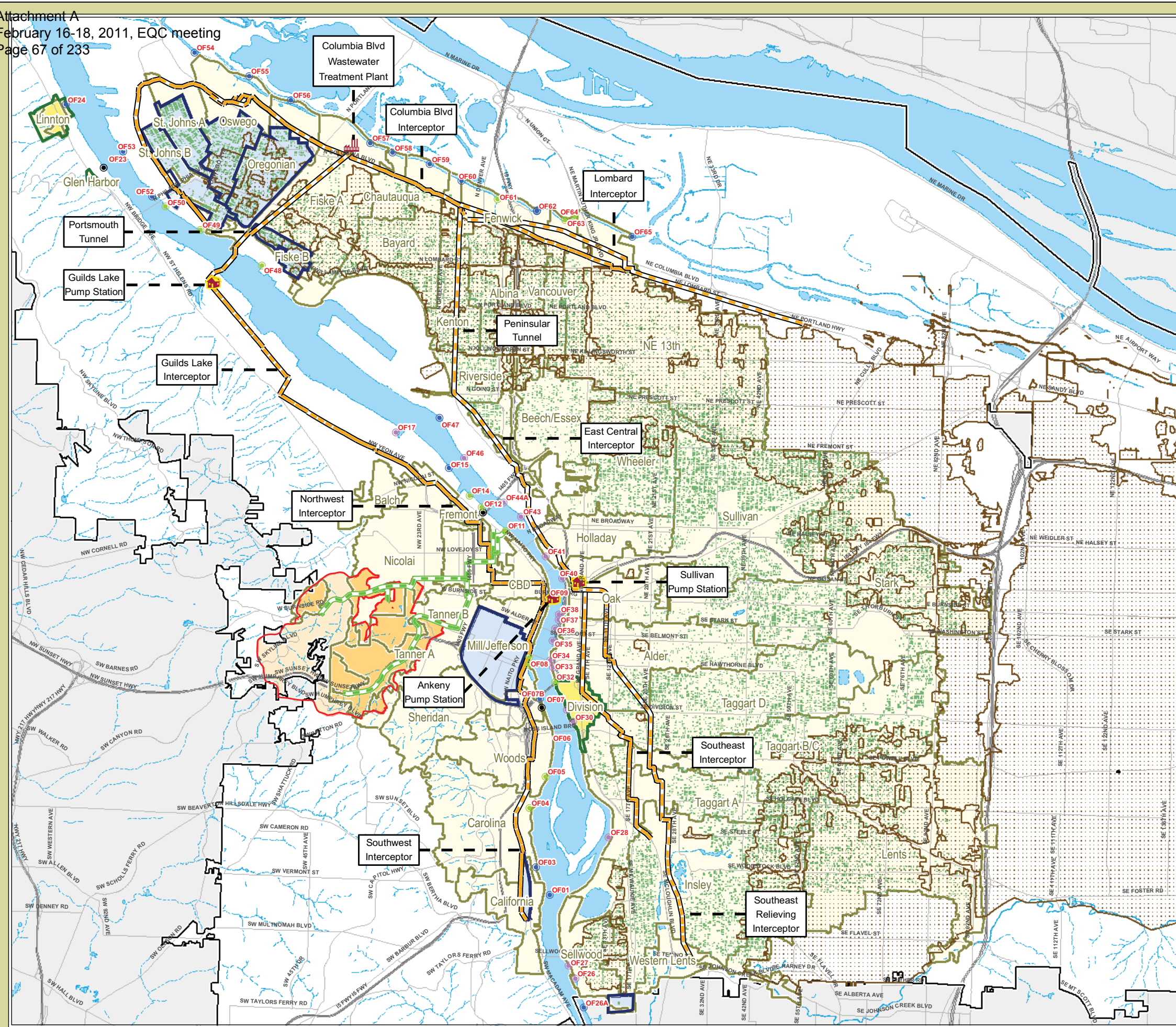
Figure 3-4 Combined Sewer System and Cornerstone Projects
