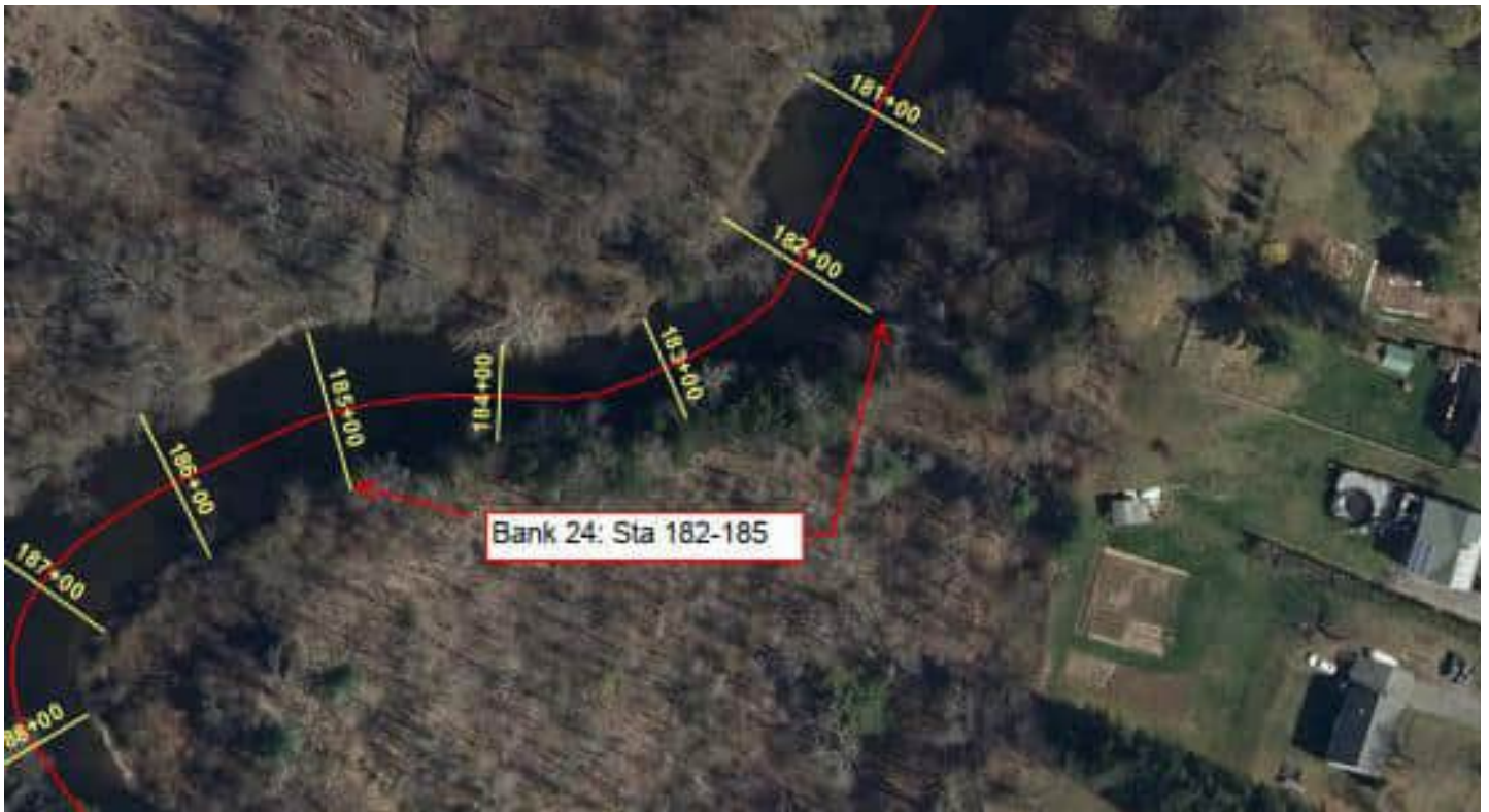
Bank 24: Stations 182-185. 300-ft along Right bend.
