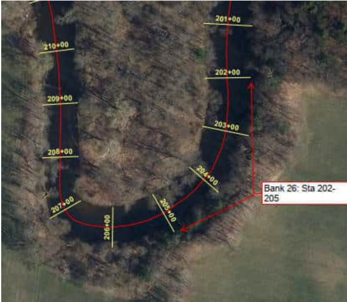
Bank 26: Stations 202-205. 300-ft stretch entering halfway around sharp right bend.
