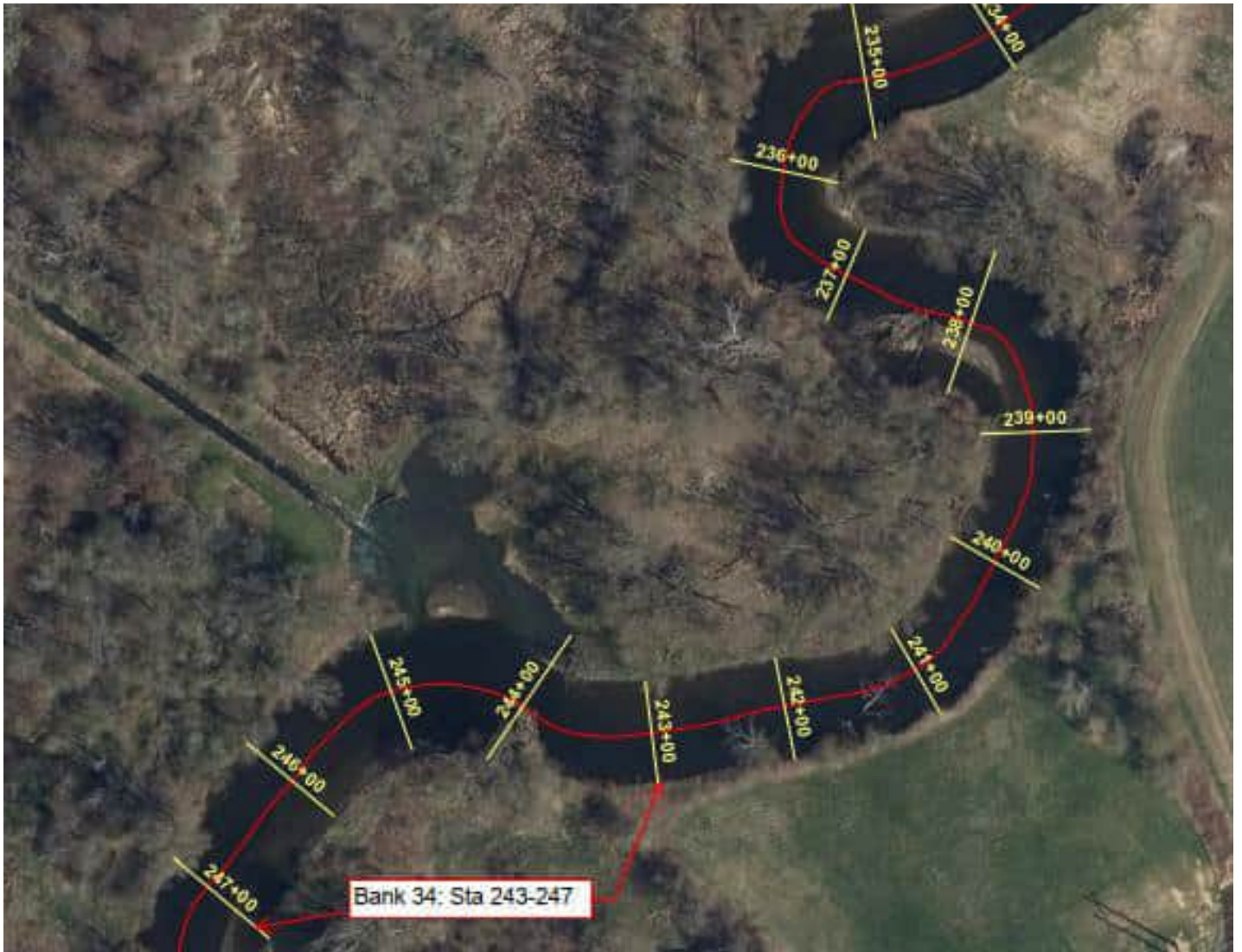
Bank 34: Station 243-247. 400-ft stretch around right to left bend. POTW discharge along right bank.
