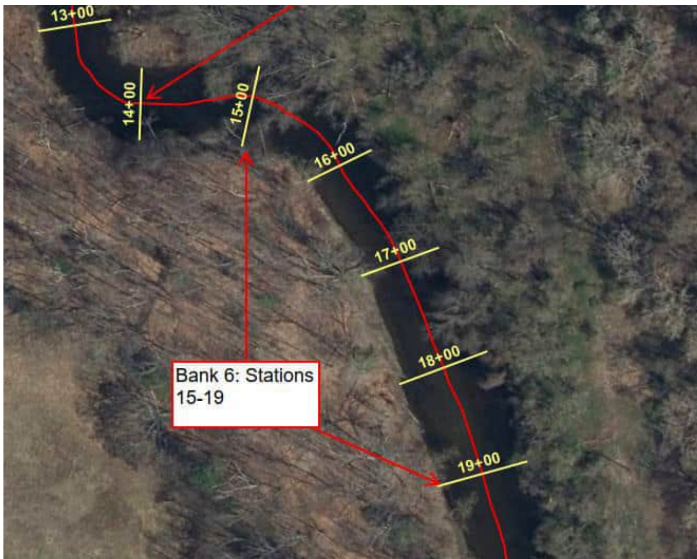
Bank 6 area: Station 15-19. 400' along Right bend at inflow from overflow channel on left bank followed by straight run.
