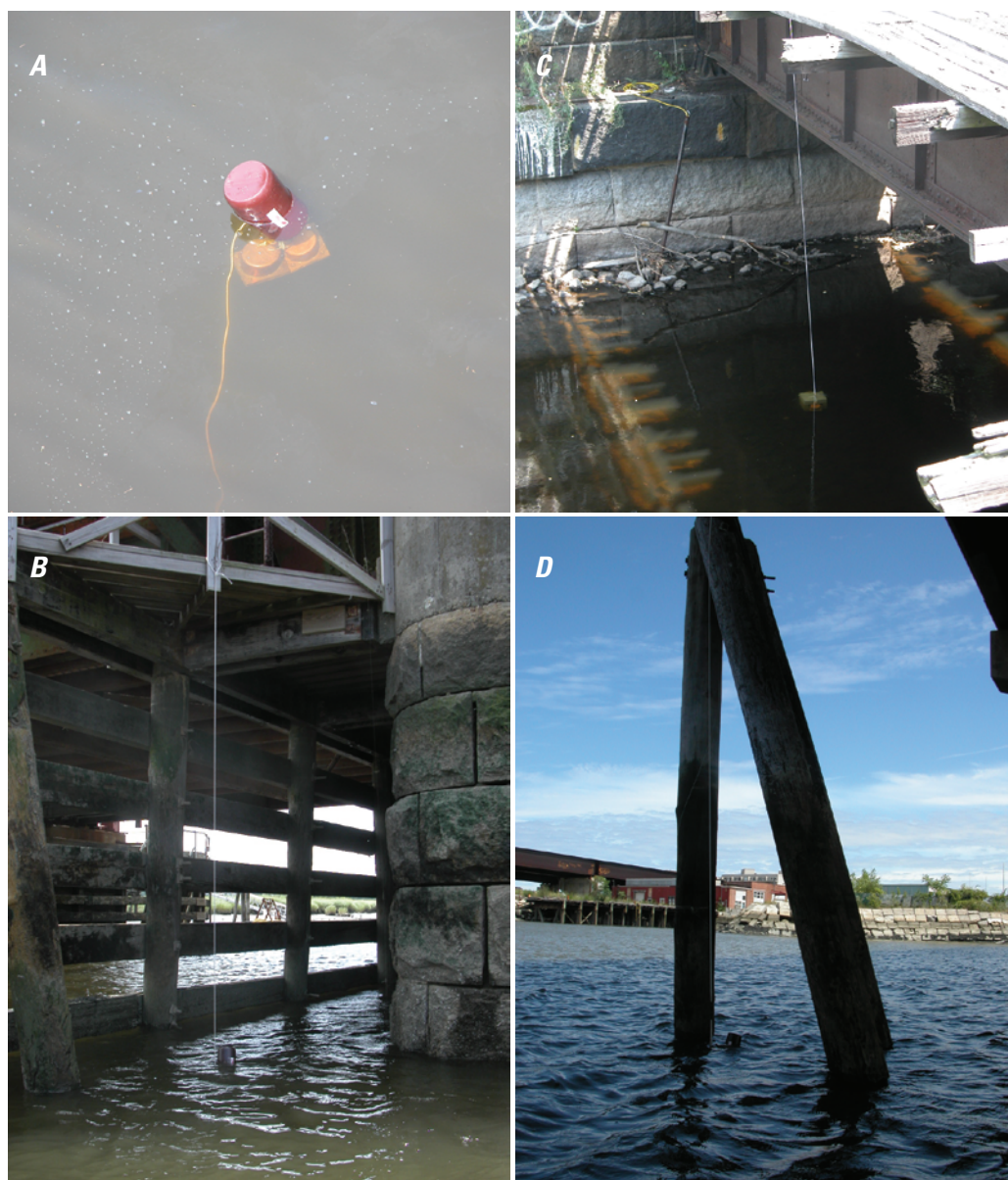
Figure 13. Passive in situ chemical-extraction samplers deployed in nontidal parts of the Neponset River and Mother Brook in (A) deep water (deeper than about 2 feet), (B) shallow water (shallower than about 2 feet) and in tidal parts of the Neponset River Estuary suspended from (C) bridges, and (D) pilings.
