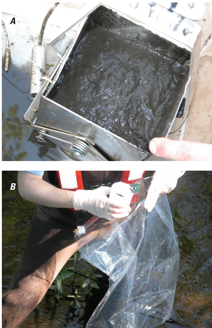
Figure 10. U.S. Geological Survey scientist collecting surficial (top 4 inches) sediment samples by means of (A) a stainless-steel dredge in water deeper than 3 feet and (B) a Teflon scoop in water shallower than 3 feet.
