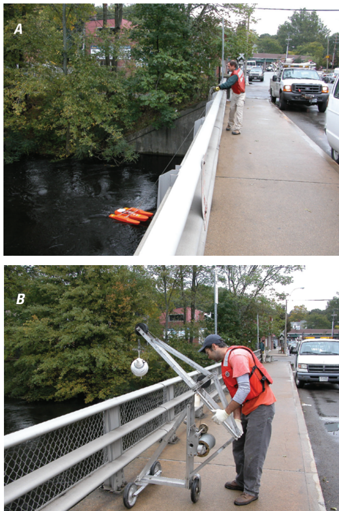
Figure 12. (A) Measurement of streamflow by means of an acoustic doppler current profiler, Blue Hill Parkway (Route 28), Mattapan and Milton, Massachusetts; and (B) U.S. Geological Survey staff collecting an isokinetic equal-width-integrated water sample with a DH-81 sampler suspended by a three-wheel base, Blue Hill Parkway, Mattapan and Milton, Massachusetts.
