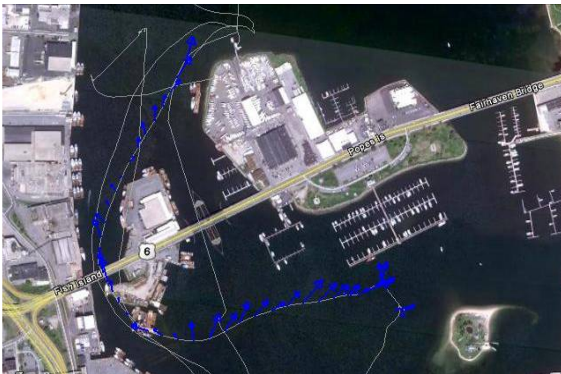
Figure 3-6. Vessel track for roving ADCP surveys of 05 Nov 2008. Track segments run between settling velocity sampling stations in lower and outer New Bedford Harbor (Figure 3-1). Velocity vectors presented are depth-averaged.
