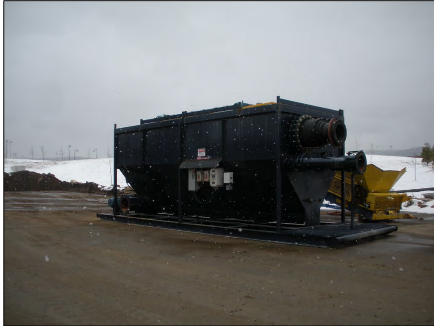
Photograph 39: Staged mixing hopper associated with hydraulic capping operations (3/22/13)
