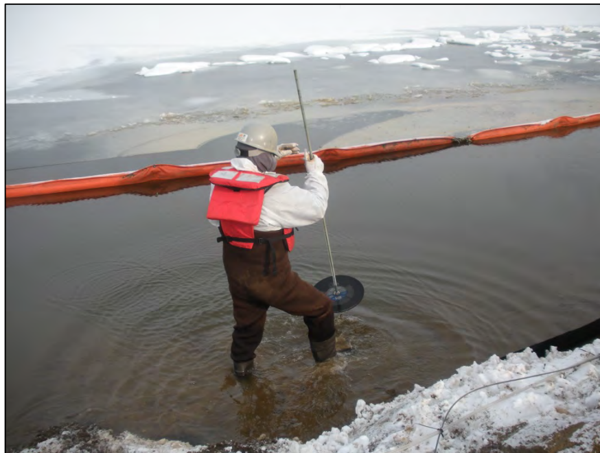
Photograph 28: Verification of thickness of near-shore restoration layer(s) (1/17/13)
