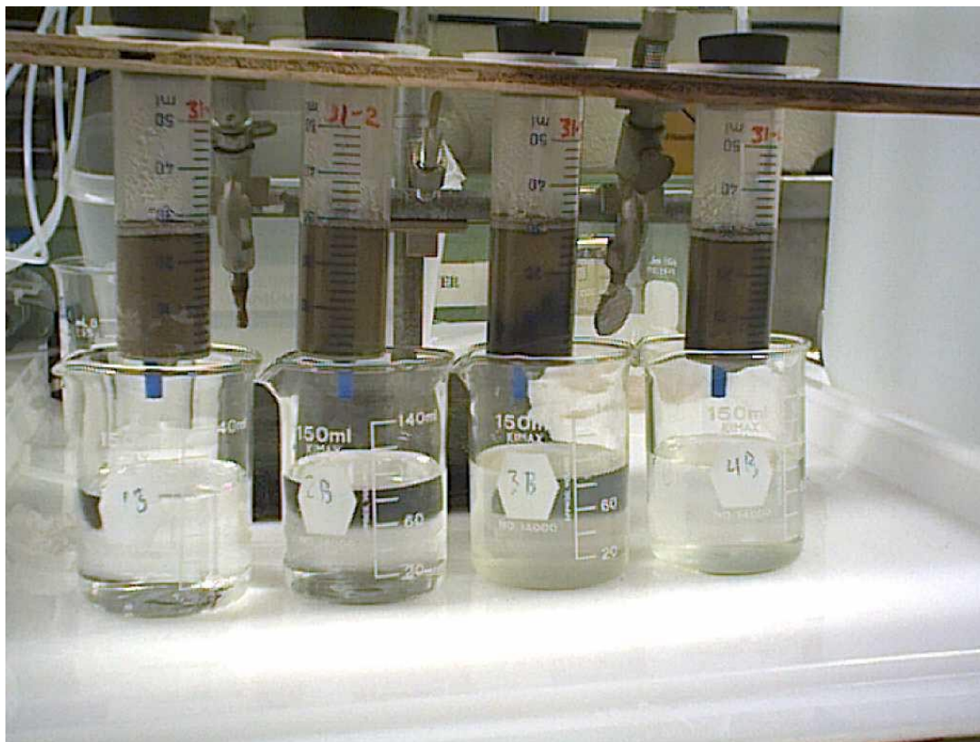
Figure 53. Illustration of Soil Column Elution. This photograph was taken during the collection of Eluate Fraction #60 from experiment “Series 31”. At this time, a total of ~ 125 bed volumes had been eluted from the columns.
