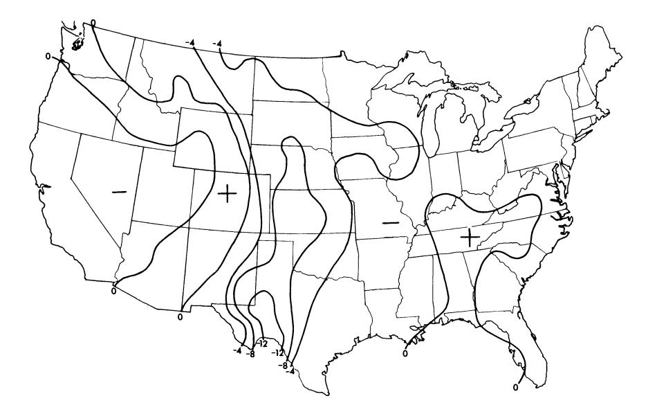
Figure 7--Deviation in inches of May-October free water surface evaporation  $E_{mf}$  (computed using meteorological factors) from equivalent map points  $E_{m2}$  (station point values from map 2) derived from the analysis of observed values. Map value =  $E_{mf} - E_{m2}$
