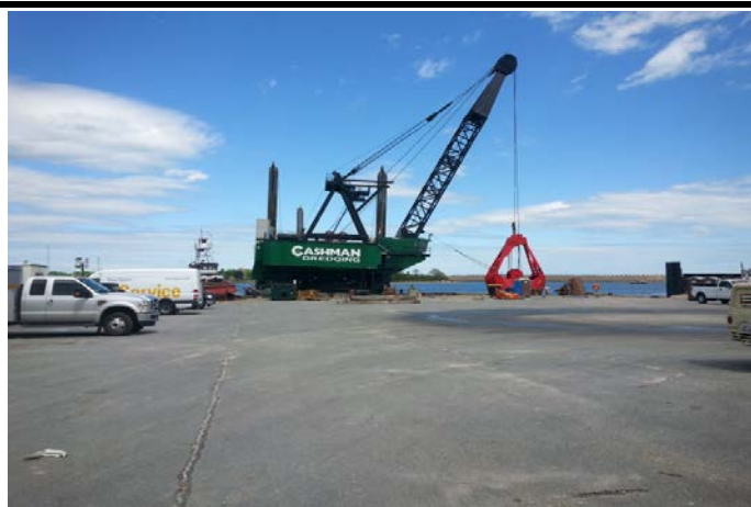
Dredge plant Dale Pyatt testing the bucket, wires, and generator.
