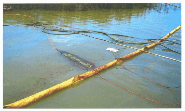
Figure 3: Floating EMA sorbent.
