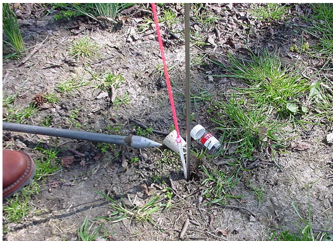
Figure D-3. Installing a passive soil gas module.
