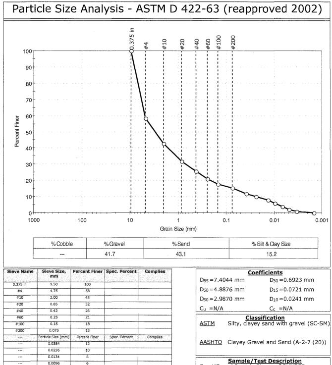
Sand/Gravel Particle Shape : ROUNDED Sand/Gravel Hardness : SOFT
