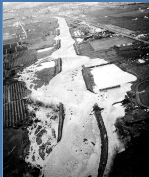
Straightened Walla Walla River in Washington Returns to Meandering Stream During Major Flooding
