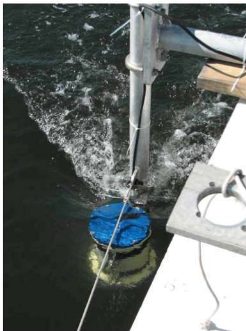
Figure 2. ADCP Mounted in Operational Position Over the Side of the Sea Quest with the Acoustic Transducers Just Below the Water Surface.
