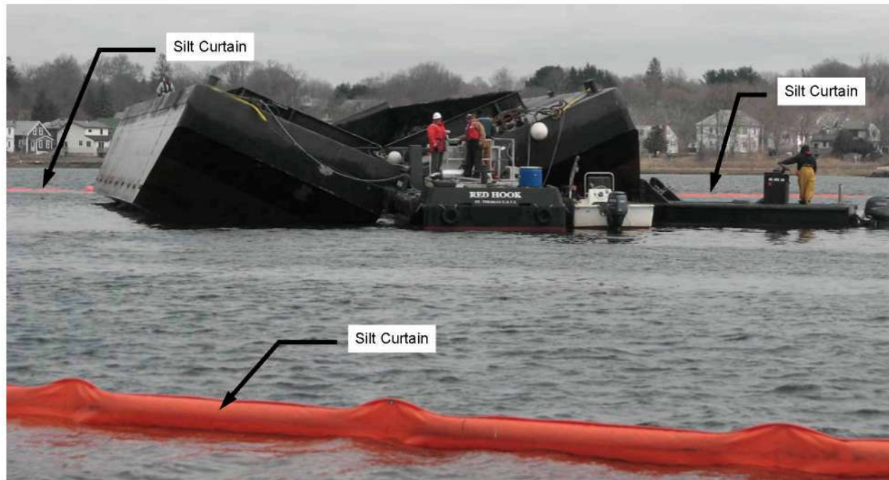
Figure 4. Split Hull Scow Immediately after Placement of Dredged Material into the CAD Cell.
