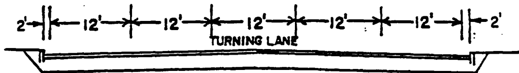
TYPICAL SECTION WITH 12' TURNING LANE ( WHERE NECESSARY )
