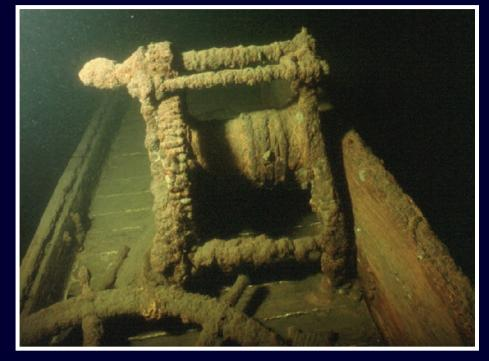
Steering mechanism located near the steering wheel
