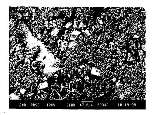
M1 210X Robinson Backscattered Electron (RBSE) micrograph of solid waste from the west leg of the northwest trench, showing typical fresh material. EDS spectrum 38001A was averaged over this field of view.
