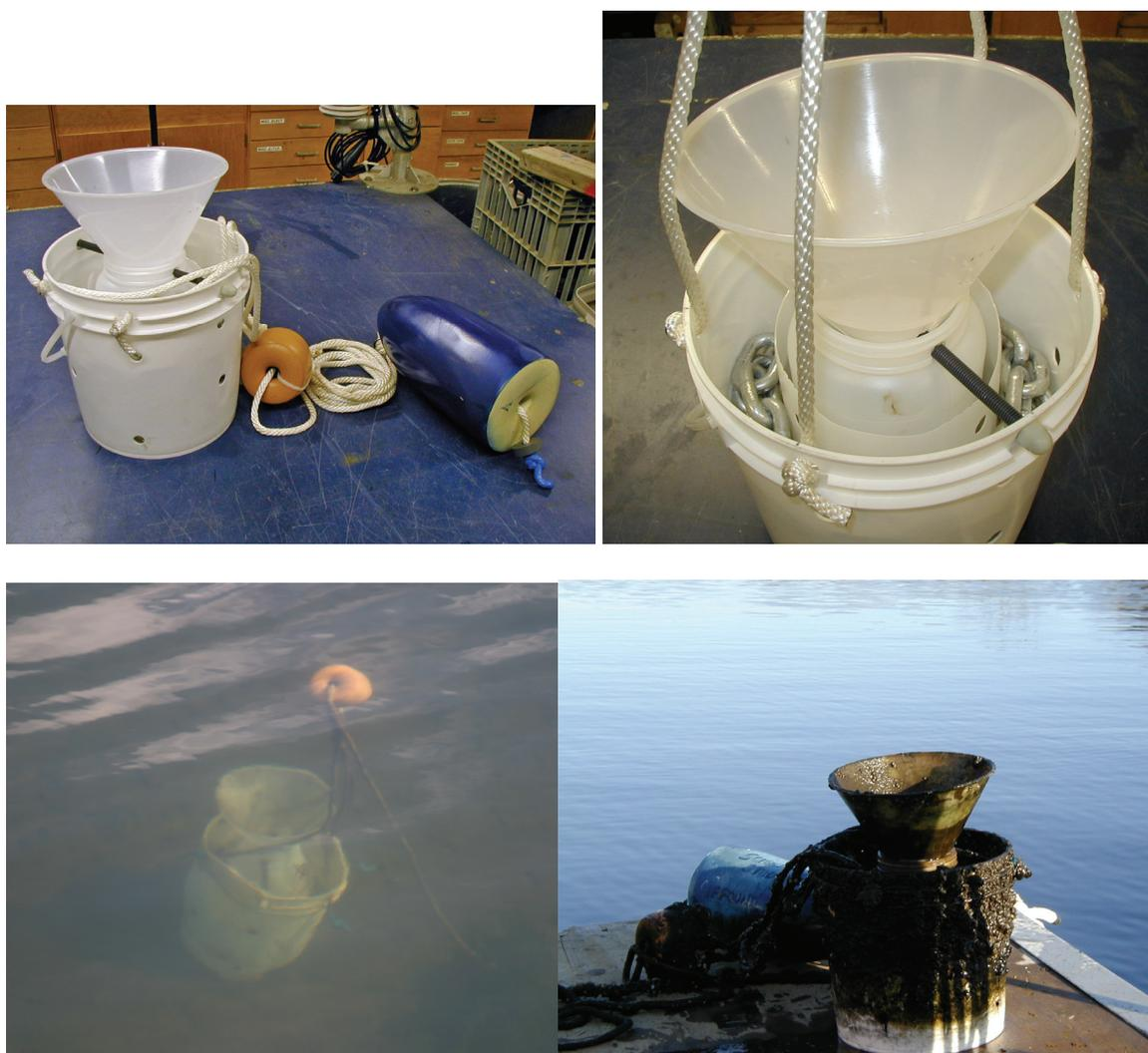
Figure 5. Pictures of Sediment Traps before Deployment (Top), During Deployment (Bottom), and Recovery (Bottom).
