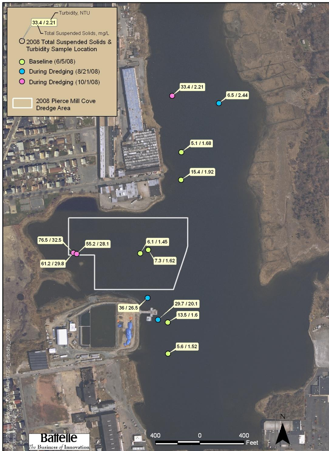
**Figure 14. Total Suspended Solids and Turbidity Results in Site Water Samples Collected Prior to and During Dredging Activities.**
