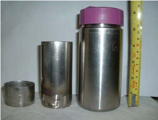
Photo 1. In order from left to right: Ring which supports crucible, Crucible, and centrifuge tube. All are composed of stainless steel. The crucible is placed on top of metal ring inside of the centrifuge tube during centrifugation of the sample
