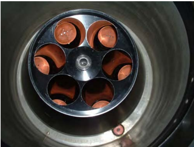
Photo 3. View from above. The inside of the centrifuge, showing 6 centrifuge tube compartments.
