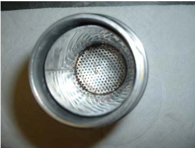
Photo 2. View from above. The ring and crucible inside of centrifuge tube. Can see the perforated bottom of crucible.
