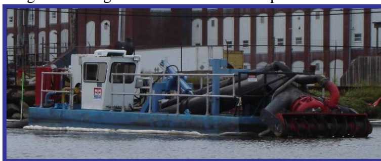
Figure 9. Mud Cat TM Hydraulic Dredge.
