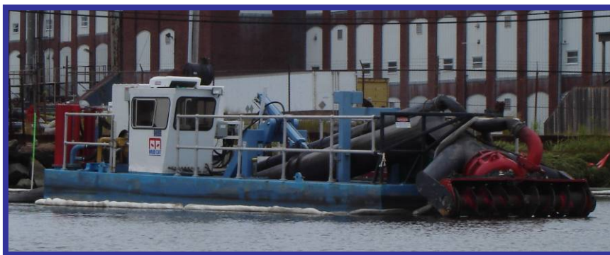
Figure 9. Mud Cat™ Hydraulic Dredge
