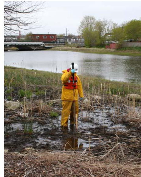
Figure 7 Impact Driven Push Core Soil Sampling Device Used for Short Cores
