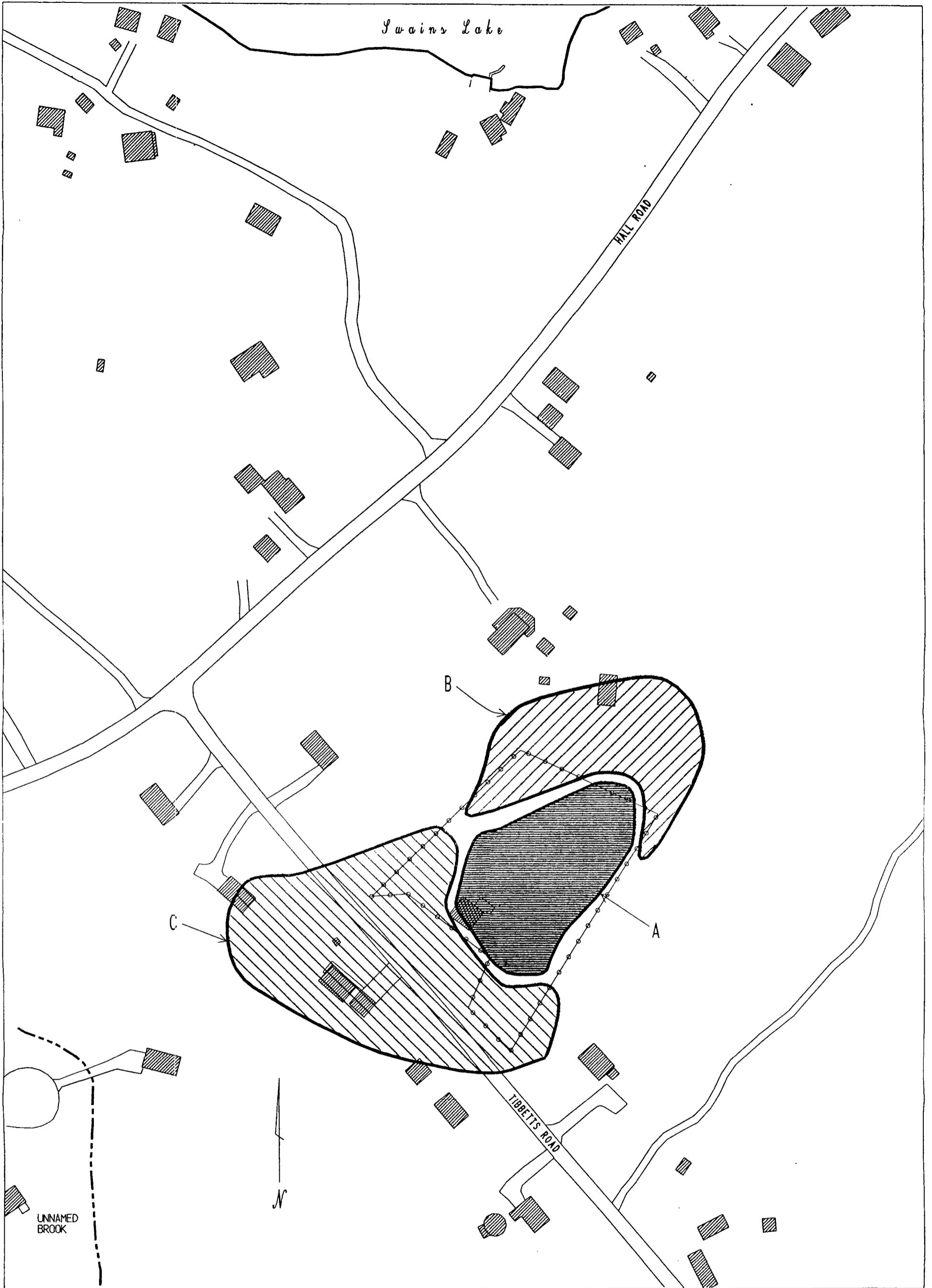
Figure B-1 PRECIPITATION, INFILTRATION AREAS IN OVERBURDEN FOR FLUSHING CALCULATIONS TIBBETTS ROAD, BARRINGTON, NH
