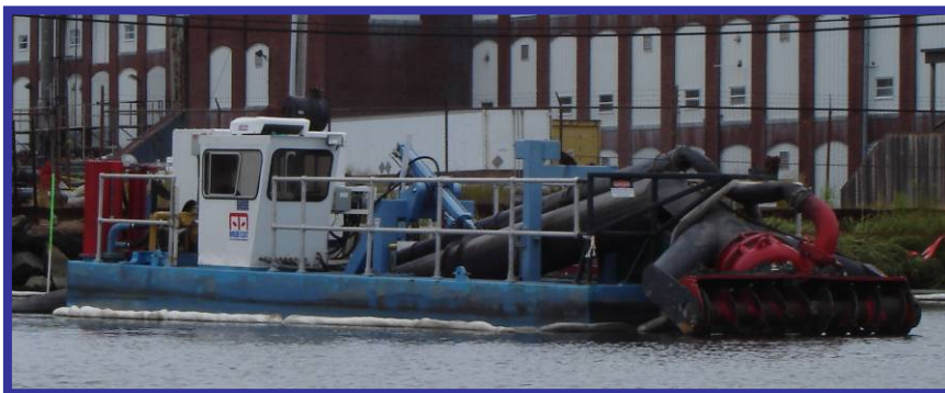
Figure 9. Mud Cat™ Hydraulic Dredge
