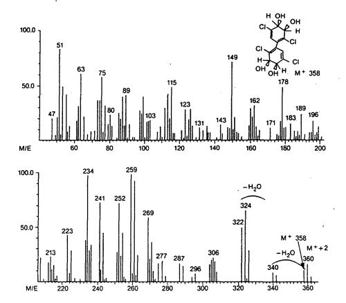
Figure 1-2. Mass spectrum of a metabolite of the cis-3,4-dihydrodiol of 2,5,2',5'-CB. This compound, which eluted at scan number 450 of the GC analysis, has been identified as the bis-3,4-dihydrodiol of 2,5,2',5'-CB.
