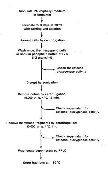
Figure 3-1. Flow chart for the preparation of cell-free fractions with PCB-degrading activity.
