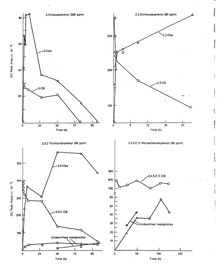
Figure 7-3. Time course of PCB degradation and metabolite production in moist soil inoculated with resting cells of *P. putida* LB400.
