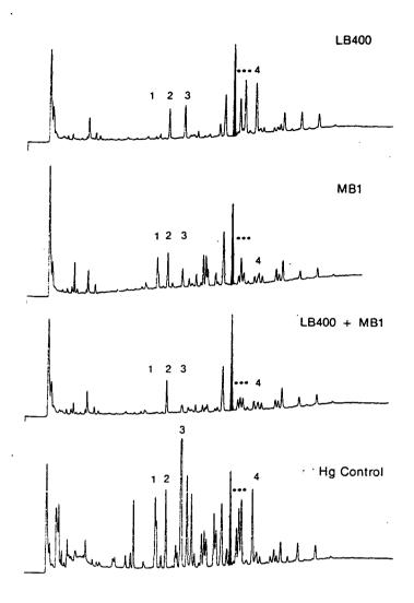
Figure 7-1. Biodegradation of soil-bound Aroclor 1242 by MB1 and LB400 applied separately or as a mixture. Soil spiked with 50 ppm of Aroclor 1242 was incubated with resting cells for 3 days. Cells (2 ml at approximately 109 cells/ml) were incubated with 0.4 g of soil. The shaded peak is a nondegradable PCB congener used as an internal standard.
