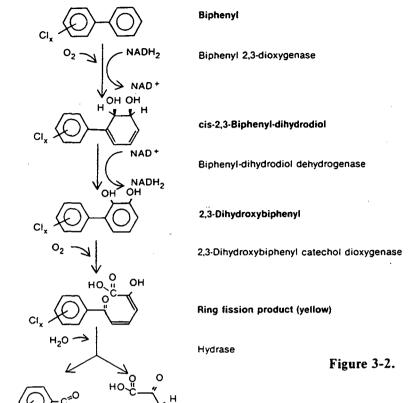
Figure 3-2. Degradation of biphenyl and PCBs by the biphenyl 2,3-dioxygenase pathway.
