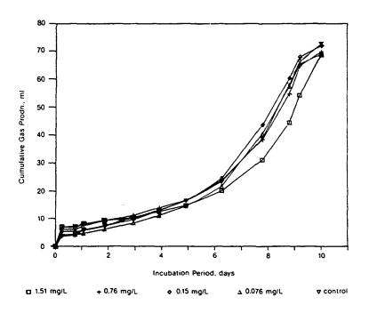
Figure 9-2. Anaerobic toxicity assay results for 2,3,4,6-tetrachlorobiphenyl.
