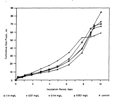
Figure 9-1. Anaerobic toxicity assay results for 2,4,6-trichlorobiphenyl.
