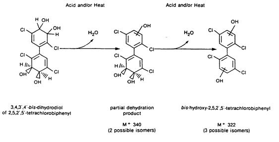
Figure 1-3. Proposed dehydration mechanism of the bis-3,4-dihydrodiol of 2,5,2',5'-CB.
