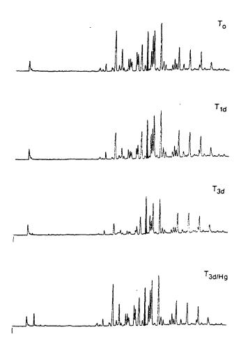
Figure 7-2. Biodegradation of PCBs in an environmental sample by Pseudomonas putida LB400. Cells (2 ml at approximately 10° cells/ml) were incubated with 0.2 g of soil from dragstrip site 43C (described in the text). The shaded peak is a nondegradable PCB congener used as an internal standard.
