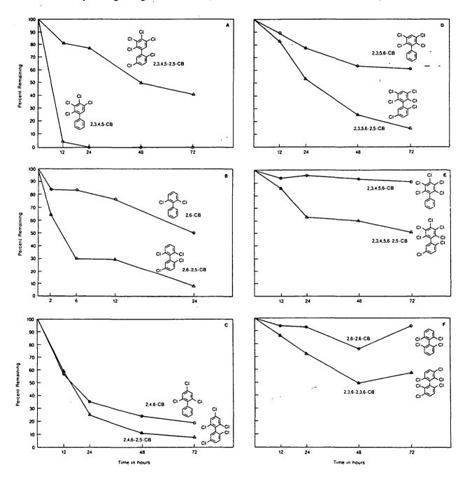
Figure 2-1. The effect of 2,5-chlorine substitution on PCB degradation in H850.
