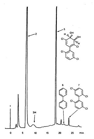
Figure 1-1. HPLC analysis of the transformation products of 2,5,2',5'-tetrachlorobiphenyl. Fifteen mg of 2,5,2'5'-CB were incubated with resting cells of H850 for 8 hours. Peaks 1-4 are polar products.
