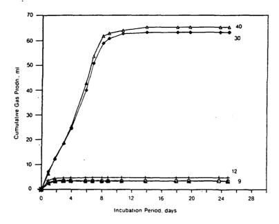
Figure 9-5. The effect of octylphenol Triton surfactants (333 mg/liter) on the anaerobic biodegradation of acetate.
