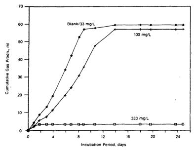
Figure 9-3. The effect of Triton X-100 on the anaerobic biodegradation of acetate.
