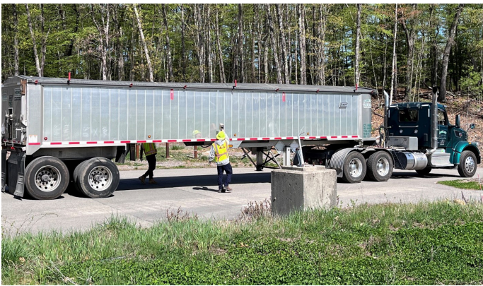
Photo 9: In order to protect site workers, truck drivers, and the community, the outside of each truck is scanned for radiation prior to leaving the site.
