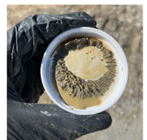
Microscale zero-valent iron (mZVI) particles present on jar lid
