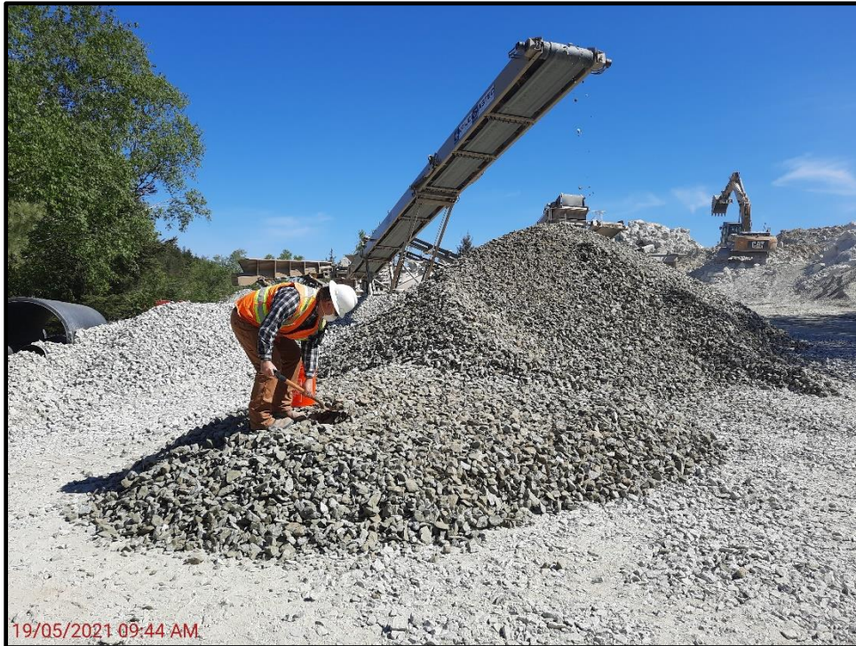
Photo 1. View of sample collection for testing at the rock processing plant. (see attached Figure E-1 for location of processing area)
