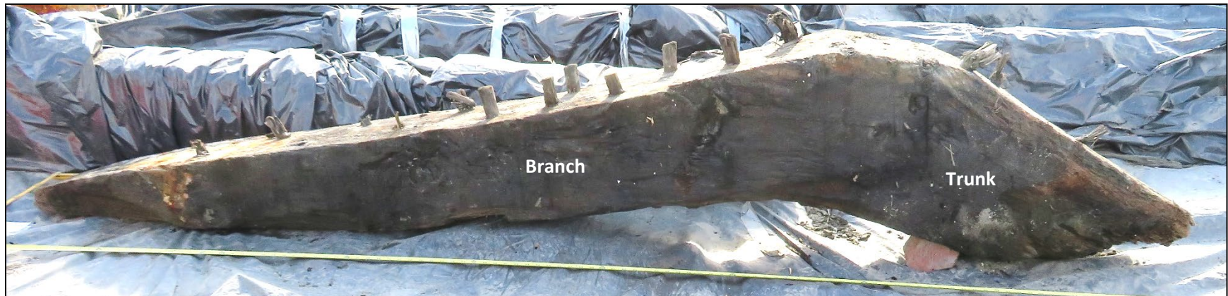
Figure 17. Examination of the surfaces, shapes, and wood grain of NBHSS UAD SW#3's framing timbers revealed several were "rough cut" and retained their source-tree's naturally rounded surfaces and shapes (upper image), and many were fashioned from "compass timbers" that were cut from parts of trees that were selected because their naturally grown shape fit the desired design shape of a particular timber (lower image) (photographs by David Robinson, DSRA).
