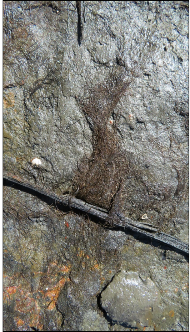
Figure 21. Tarred animal hair “felting” and sheathing nail holes on the exterior surfaces of NBHSS UAD SW#3’s hull planking and keel provided evidence that the vessel’s hull had once been sheathed in protective sacrificial wooden hull sheathing (photographs by David Robinson, DSRA).
