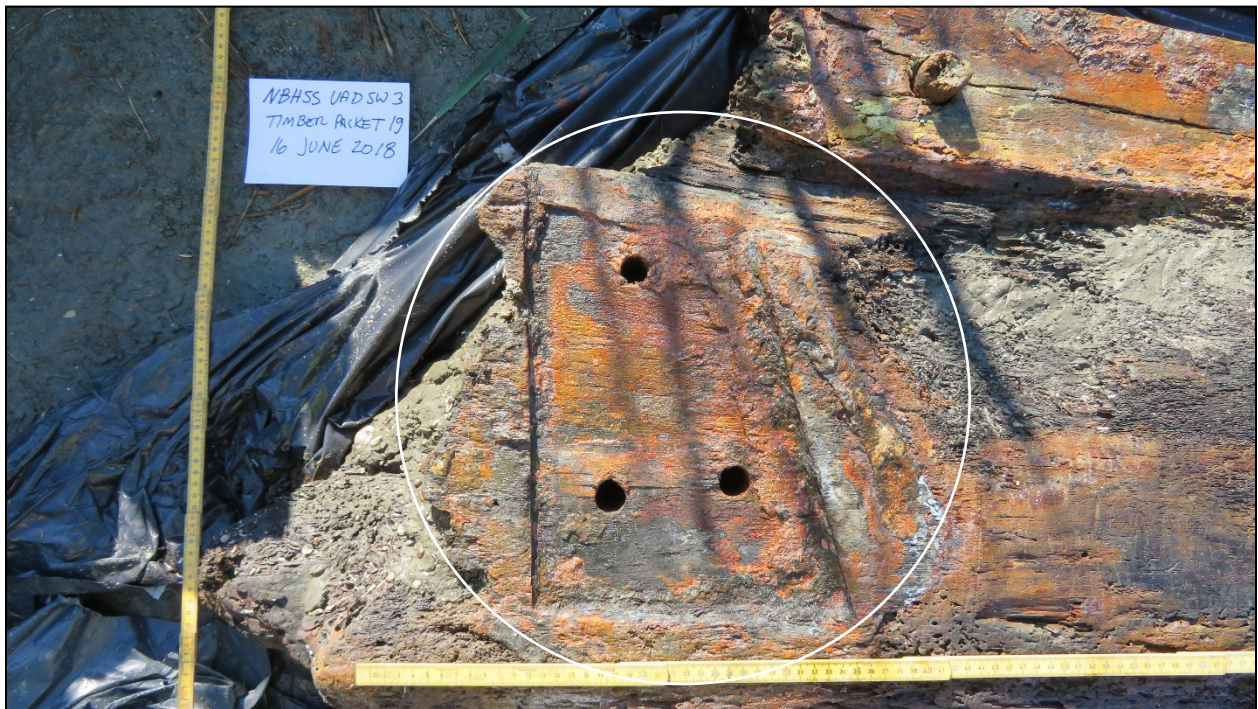
Figure 16. Corrosion-stained recesses or “mortises” cut into both sides of the aft end of the keel once held the lower half of vertically-oriented iron “fishplates.” These through-bolted iron plates extended up the sides of the keel and onto the sides of the lower portion of the sternpost and helped secure the connection between the bottom or “heel” the sternpost and the top surface of the keel’s aft end (photographs by David Robinson, DSRA).
