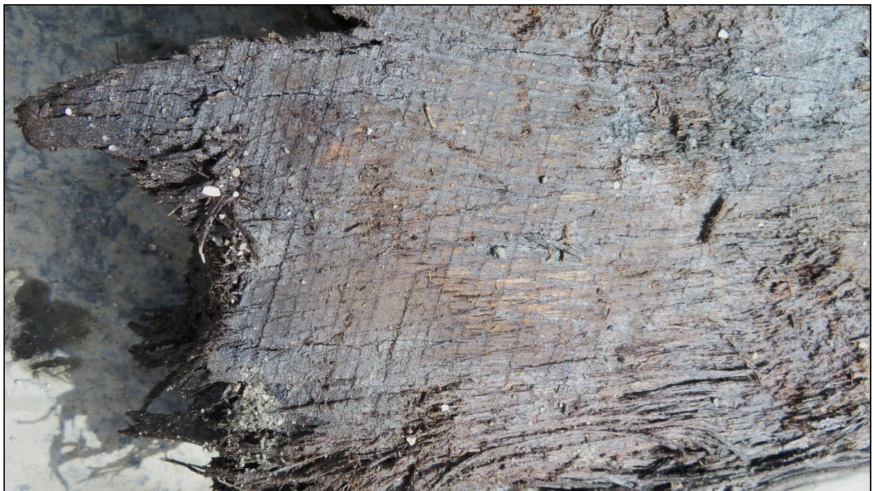
Figure 20. Surface features observed in NBHSS UAD SW#3's hull planking were limited to a single roman numeral scribe-mark ("X") near the intact end of one of the non-garboard hull planking fragments (upper image), and saw kerf marks that were clearly associated with a large circular saw (upper and lower images). Introduced in the 1830s, circular saw blades were commonly used in the sawmills of the eastern United States by the middle 1800s, but were introduced and adopted in English sawmills significantly earlier (i.e., the late 1700s) (photographs by David Robinson, DSRA).
