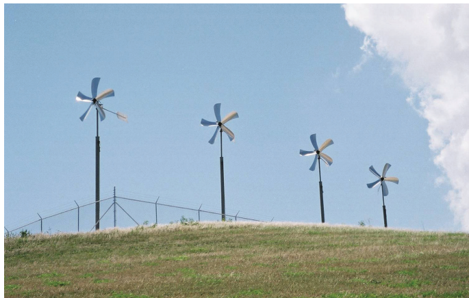
Windmills power equipment to remove oil from contaminated groundwater.
